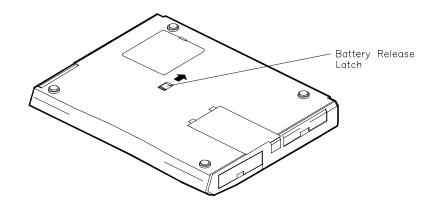
Figure Section 2-5 Battery Release Latch Location
