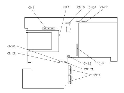
Figure Section 4-1 System Board Connector Locations
