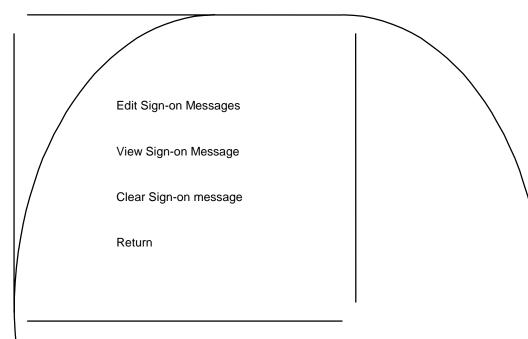
The edit option creates or changes a custom sign-on message. This sign-on message can be up to 40 characters and is displayed every time the system boots. View shows the sign-on message, if any, that will be installed into the new BIOS. The clear function erases the custom sign-on message. Exit returns to the Main Menu.
