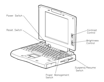
Figure Section 2-2 Control and Switch Location
