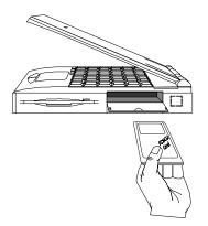
Figure 1-6 Inserting a PCMCIA Card
