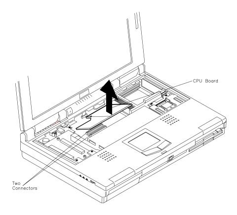
Figure 4-7 Removing the CPU Board
