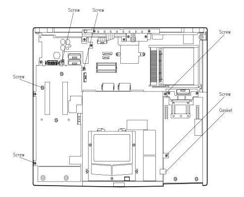
Figure 4-12 Removing the CD-ROM Reader Assembly Screws
