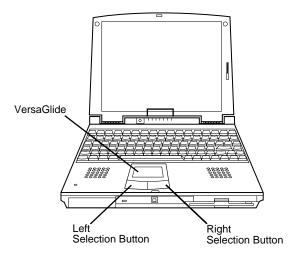
Figure Section 1-4 VersaGlide Location
