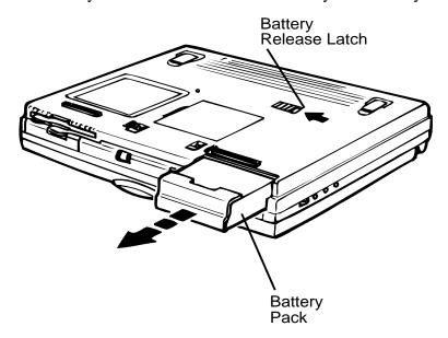
Figure 4-1 Releasing the Battery Pack
