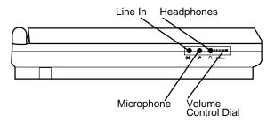
Figure Section 1-6 Left Side Features
