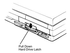
Figure 4-2 Removing the Hard Disk Drive (Step 1)
