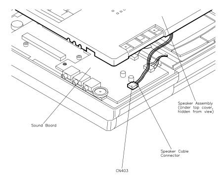
Figure 4-9 Removing the LCD Assembly (Step 2)
