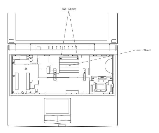
Figure 4-6 Removing the Heat Sink/Shield Subassembly
