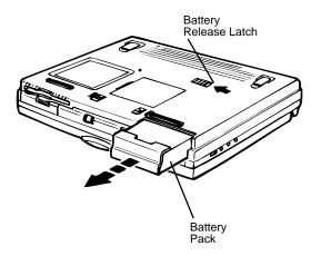
Figure 2-5 Battery Release Latch
