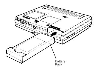
Figure 2-6 Inserting Battery Pack
