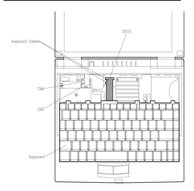
Figure 4-5 Removing the Keyboard
