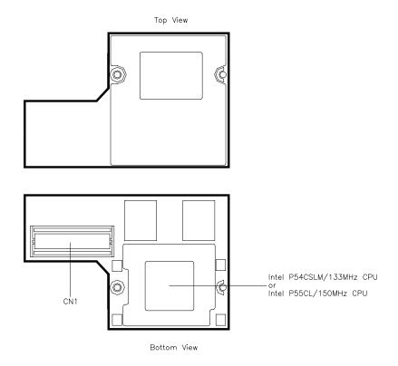
Figure Section 1-8 CPU Board Layout
