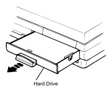
Figure 4-4 Remove Hard Disk Drive (Step 3)
