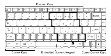
Figure Section 1-3 Keyboard Layout
