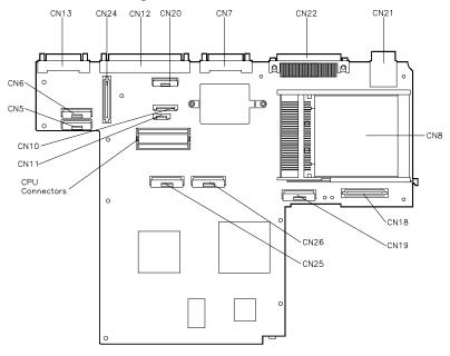
Figure Section 1-10 I/O Board layout
