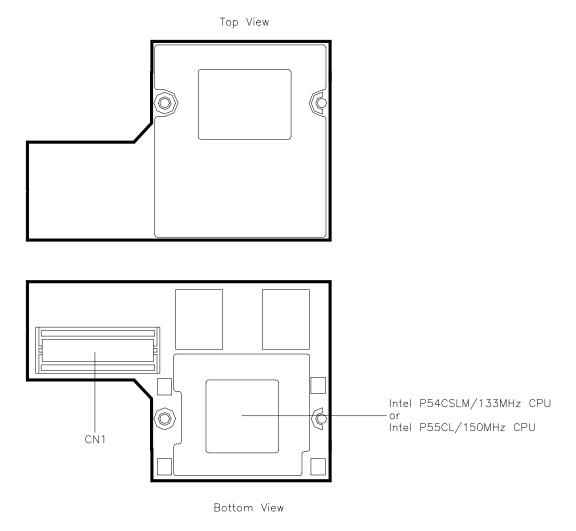
Figure A-1 CPU Board Layout
