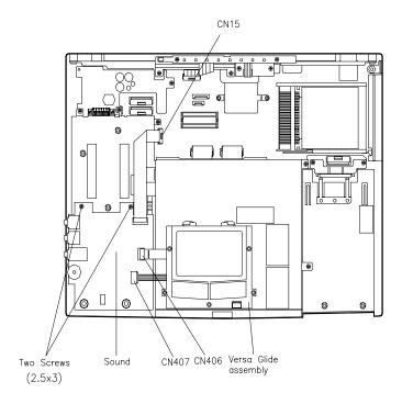
Figure 4-10 Disconnecting the VersaGlide Cables
