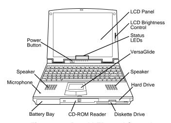
Figure 2-7 Panel LEDs and Controls
