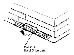
Figure 4-3 Removing the Hard Disk Drive (Step 2)
