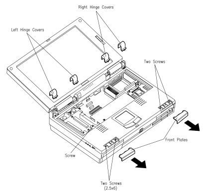
Figure 4-8 Removing the LCD Assembly (Step 1)
