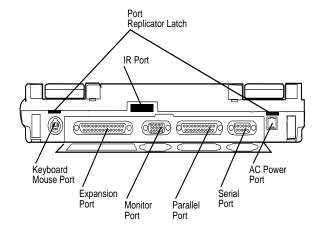
Figure 2-3 Power and I/O Connector Locations
