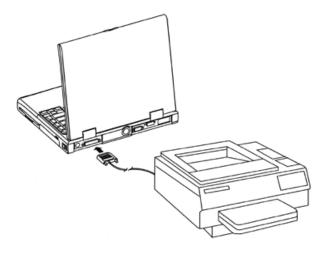
Figure 1-15 Connecting to the Printer Port
