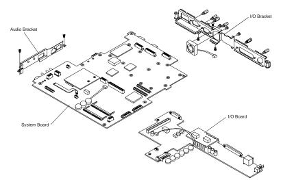
Figure 5-11 The Electronic Module Assembly
