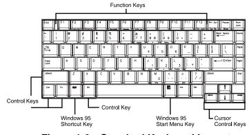
Figure 1-6 Standard Keyboard Layout
