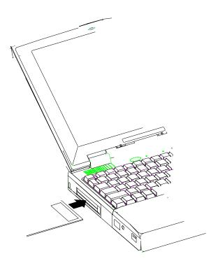
Figure 1-11 Inserting a PC Card
