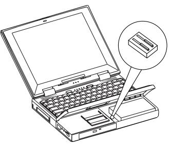
Figure 5-7 One dip switch bank
