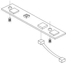
Figure 5-10 The LED Board Module Assembly
