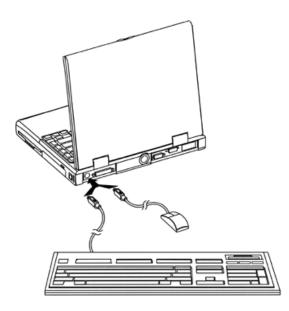
Figure 1-13 Connecting an External Keyboard and PS/2 Mouse
