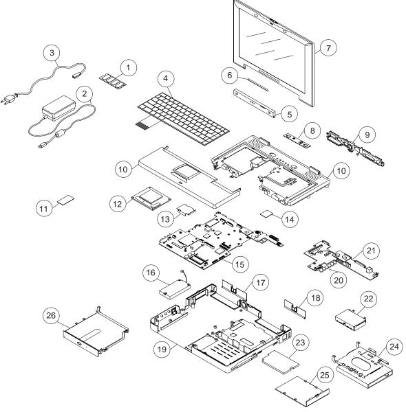
Figure 5-12 NEC Versa 2700 Series Illustrated Parts Breakdown
