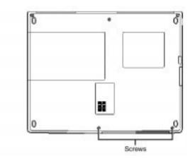
Figure 5-5 Locating the palm rest screws
