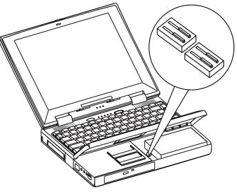
Figure 5-6 Two dip switch banks
