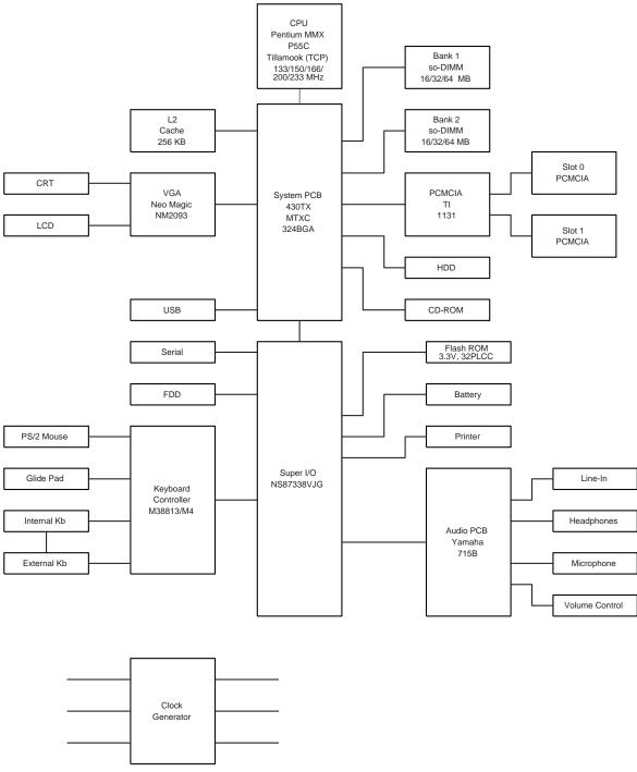
Figure 3-1 Functional Block Diagram
