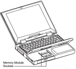
Figure 5-4 Memory module sockets
