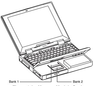
Figure 1-8 Memory Module Sockets
