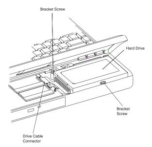
Figure 5-1 Disconnecting the Hard Drive Assembly
