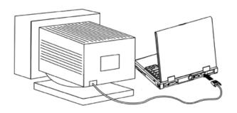
Figure 1-14 Connecting an External Monitor
