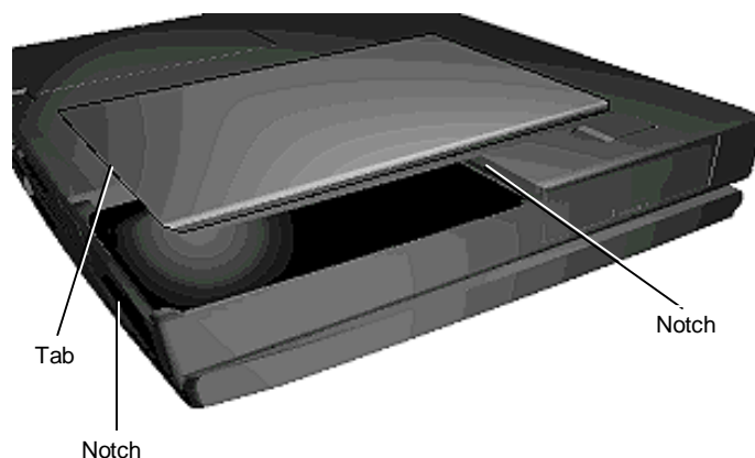
Figure Section 2-11 Battery Bay Cover Replacement
