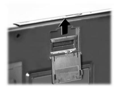
Figure 4-4 Pressing the Release Lever
