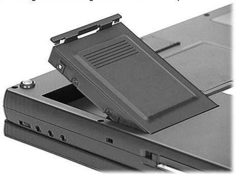
Figure 4-8 Removing the hard drive
