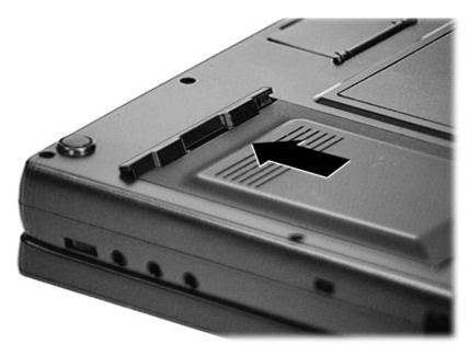
Figure 4-7 Sliding the drive towards the spacer
