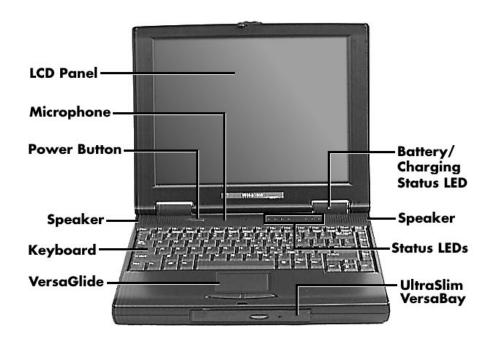
Figure 1-2 Location of Controls on the Front of the NEC Versa 5000
