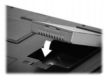
Figure 2-7 Installing the battery pack
