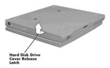
Figure 4-1 Removing the Drive Bay Cover
