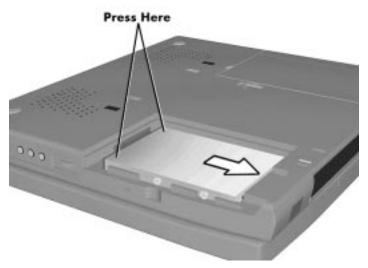
Figure 4-2 Removing the Hard Disk Drive
