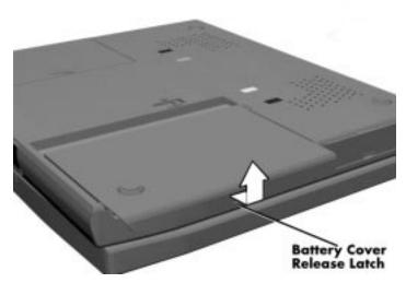
Figure 2-5 Removing the Cover
