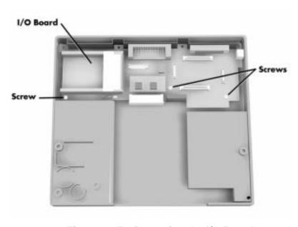
Figure 4-15 Removing the I/O Board
