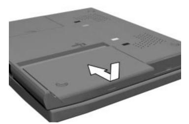
Figure 2-8 Replacing the Cover
