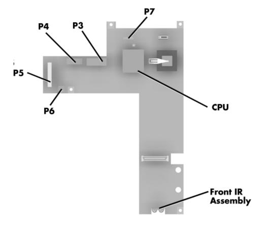
Figure A-1 CPU Board Layout
