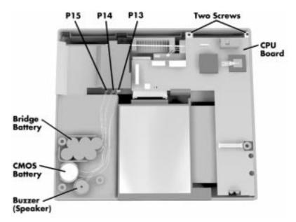
Figure 4-12 Removing Bridge Battery, CMOS Battery and Buzzer
