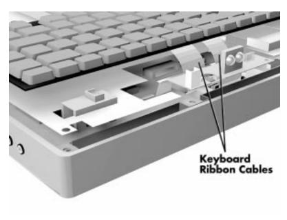
Figure 4-10 Disconnecting Keyboard Cables
