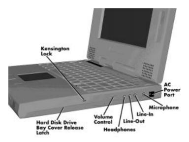
Figure 2-11 Right Side Panel Controls/Ports
