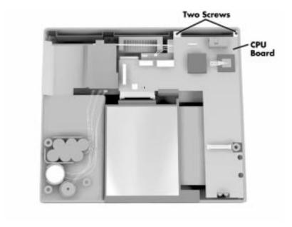
Figure 4-13 Removing the CPU Board
