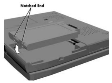
Figure 2-7 Inserting the Battery Pack
