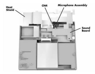
Figure 4-14 Heat Shield, Sound Board, Microphone Assembly
