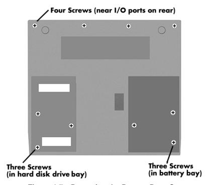
Figure 4-7 Removing the Bottom Base Screws
