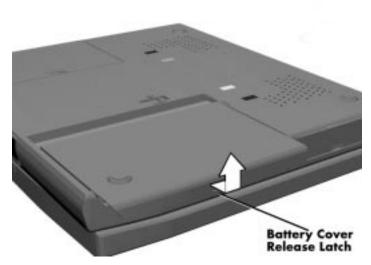
Figure 4-5 Removing the Battery Compartment Cover
