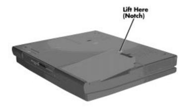
Figure 4-6 Removing the Battery
