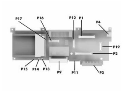
Figure 1-15 I/O Board layout
