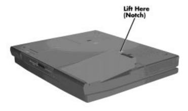
Figure 2-6 Removing the Battery
