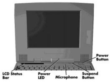
Figure 2-10 Keyboard Panel LEDs and Controls
