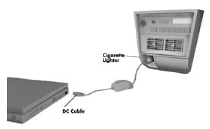
Figure 2-9 Connecting the Car DC Adapter
