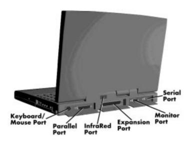
Figure 2-3 Power and I/O Connector Locations
