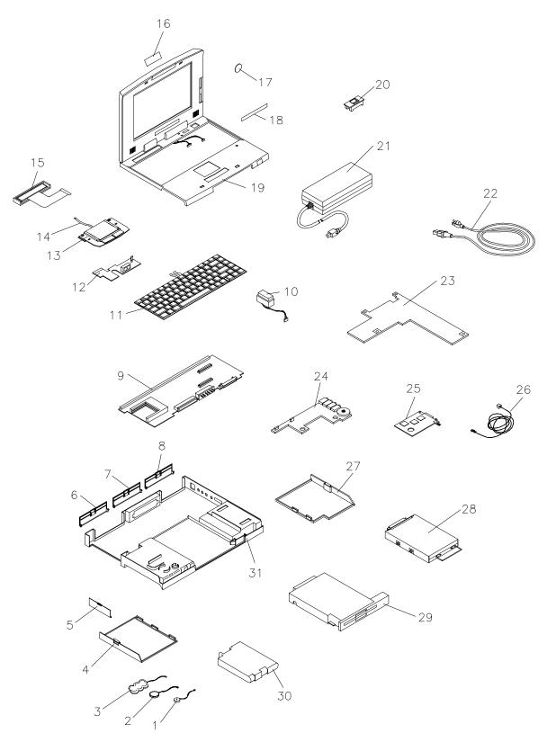
Figure 4-16 NEC Versa 6000 Ilustrated Parts Breakdown
