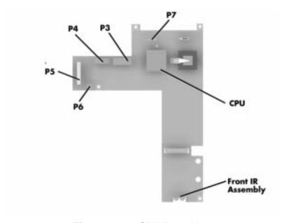
Figure 1-13 CPU Board Layout
