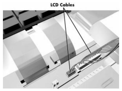
Figure 4-8 Disconnecting the LCD Connectors
