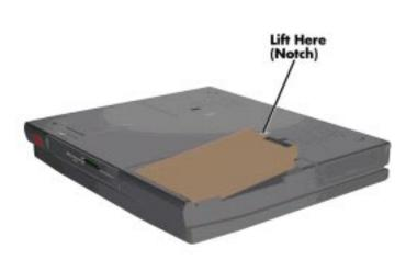
Figure 2-6 Removing the Battery
