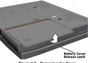
Figure 2-5 Removing the Cover
