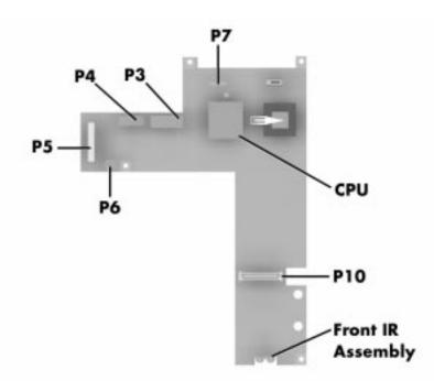
Figure 1-12 CPU Board Layout
