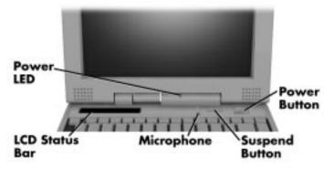
Figure 2-10 Keyboard Panel LEDs and Controls
