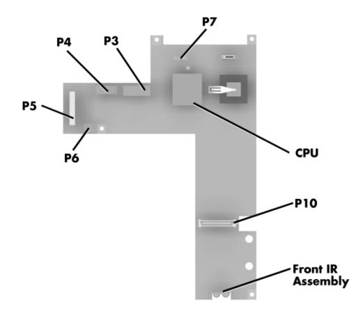
Figure A-1 CPU Board Layout
