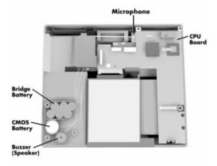
Figure 4-13 Removing the CPU Board
