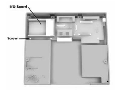
Figure 4-15 Removing the I/O Board
