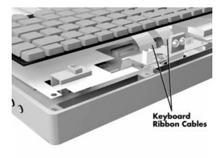
Figure 4-10 Disconnecting Keyboard Cables
