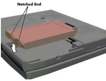
Figure 2-7 Inserting the Battery Pack
