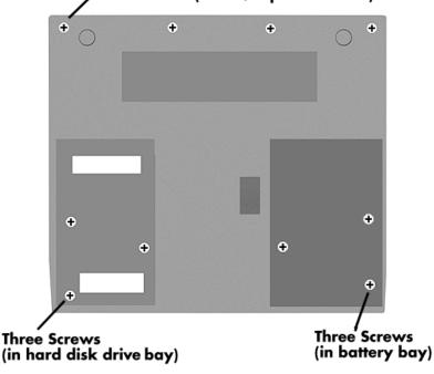
Four Screws (near I/O ports on rear)
