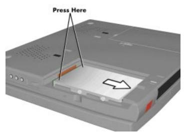
Figure 4-2 Removing the Hard Disk Drive
