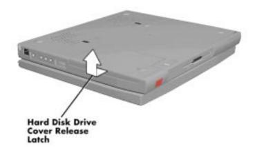
Figure 4-1 Removing the Drive Bay Cover
