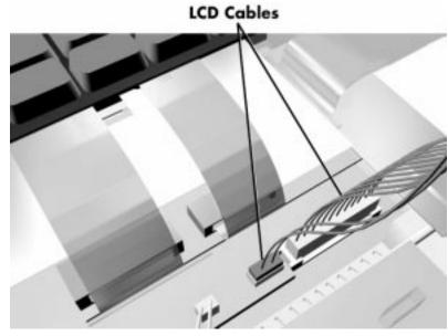
**3.** Disconnect the two LCD cables from connectors P12 and CN3 on the main board.
