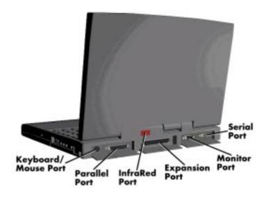
Figure 2-3 Power and I/O Connector Locations
