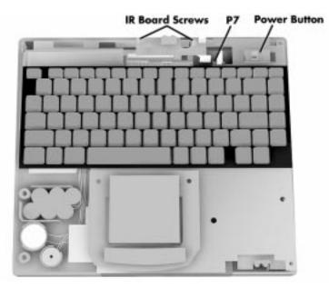
Figure 4-9 Removing the Power Button, Rear IR Assembly, Keyboard
