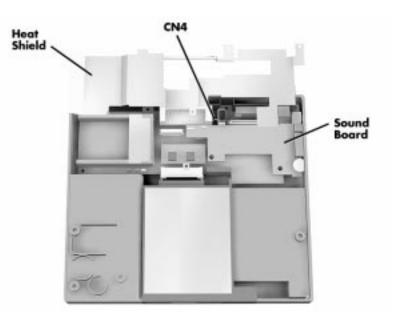
Figure 4-14 Heat Shield, Sound Board
