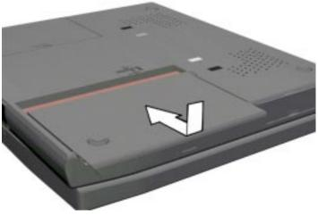
Figure 2-8 Replacing the Cover
