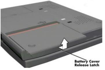
Figure 4-5 Removing the Battery Compartment Cover
