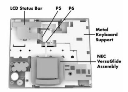
Figure 4-11 LCD Status Bar, VersaGlide Assembly, Modem Board, Metal Keyboard Supports
