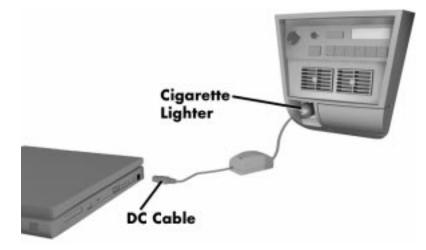
Figure 2-9 Connecting the Car DC Adapter
