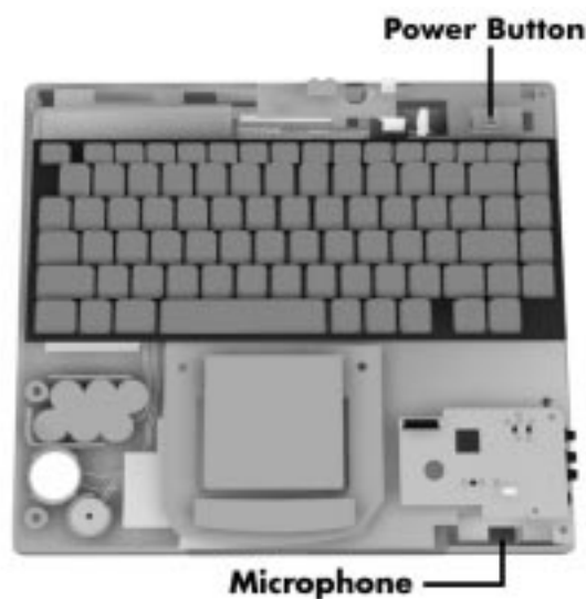
Figure 4-9 Removing the Power Button, Microphone Assembly, Keyboard
