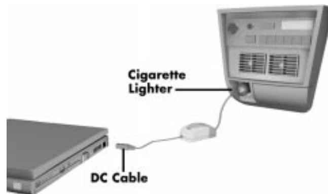
Figure 2-9 Connecting the Car DC Adapter
