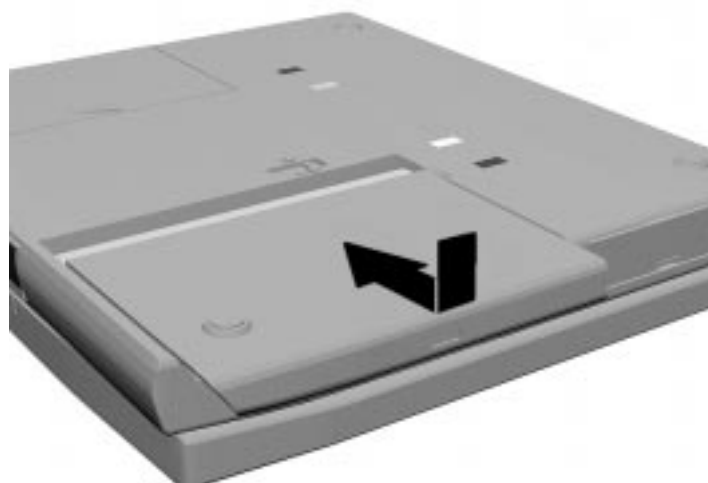
Figure 2-8 Replacing the Cover
