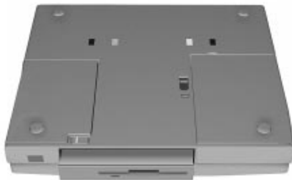
Figure 4-4 Removing the Standard Diskette Drive
