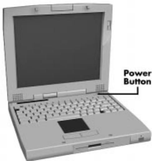
Figure 2-2 Powering on the System
