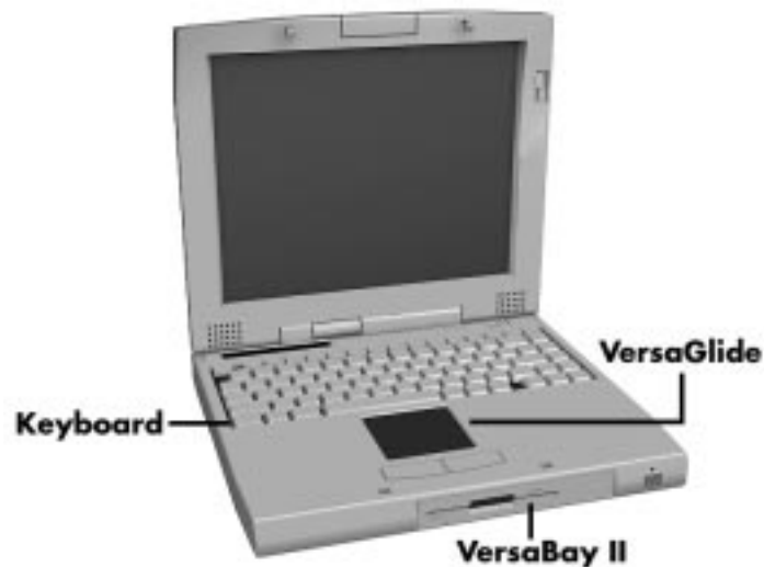
Figure 1-7 NEC VersaBay II Location
