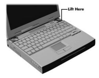
Figure 4-9 Lifting Up the Keyboard
