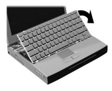
Figure 4-10 Positioning the Keyboard
