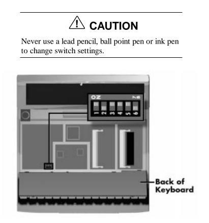
Figure 2-17 Dip Switches
