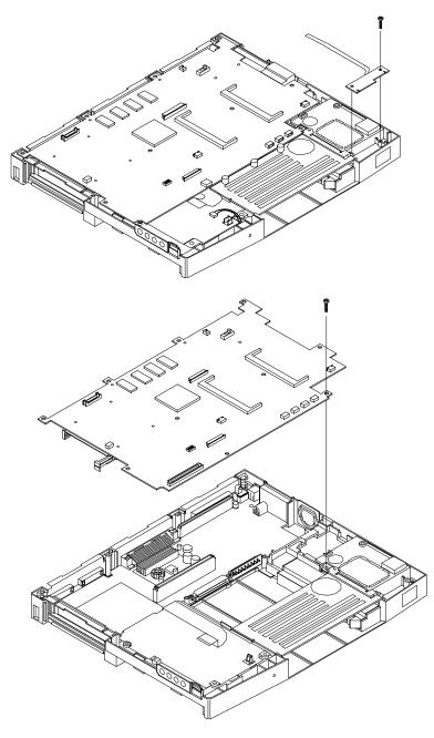
Figure 4-20 Removing IR Assembly and Graph Board
