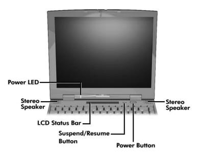
Figure 2-10 Keyboard Panel LEDs and Controls
