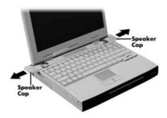
Figure 4-8 Removing the Speaker Caps
