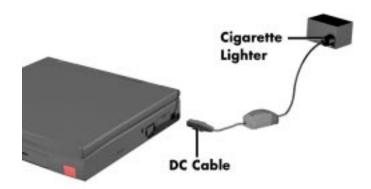
Figure 2-9 Connecting the Car DC Adapter
