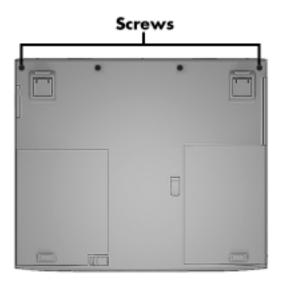
Figure 4-7 Locating the Speaker Cap Screws
