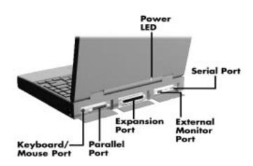
Figure 2-3 Power and I/O Connector Locations
