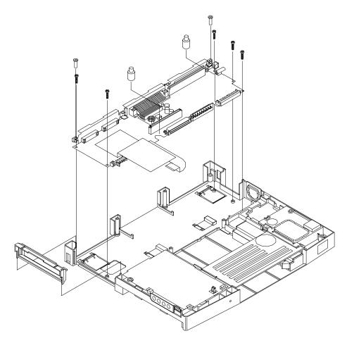
Figure 4-22 Removing the I/O Board
