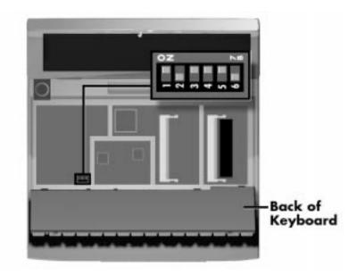
Figure 2-12 Dip Switch Location
