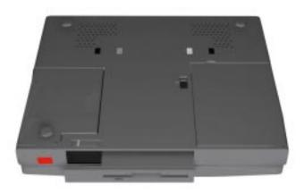
Figure 4-4 Removing the Standard Diskette Drive
