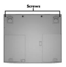
Figure 2-13 Locating the Speaker Cap Screws
