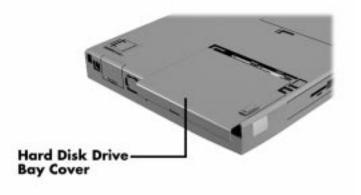
Figure 4-1 Removing the Drive Bay Cover
