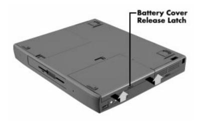
Figure 2-5 Removing the Cover
