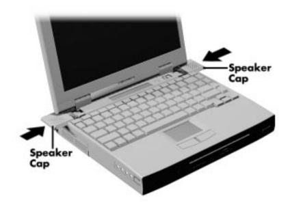
Figure 2-18 Reassembling the System
