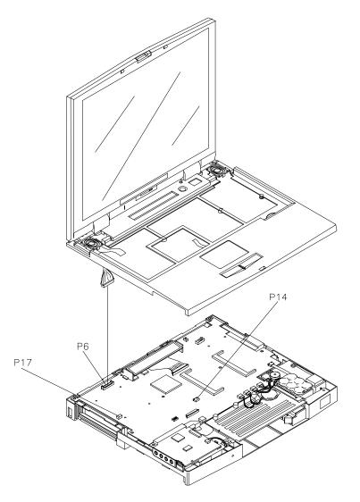
**3.** Disconnect the LCD cables from connector P6 on the Graph board. Also disconnect the speaker cables (P17) and VersaGlide cables (P14).
