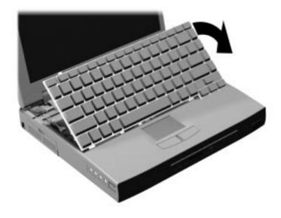
Figure 2-16 Positioning the Keyboard
