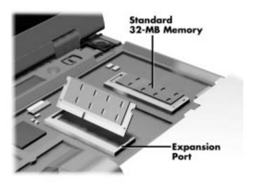
Figure 4-12 Installing the DIMM
