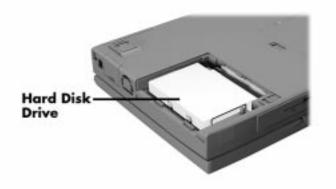
Figure 4-2 Removing the Hard Disk Drive
