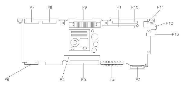
Figure 1-13 I/O Board Layout
