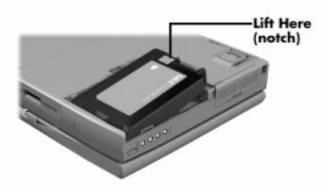
Figure 4-6 Removing the Battery
