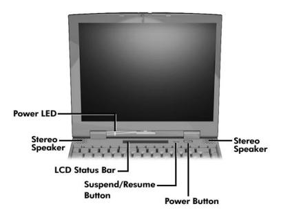
Figure 1-3 LCD Status Bar and Button Locations
