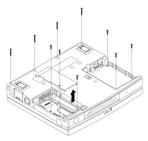
Figure 4-14 Removing the Bottom Base Screws
