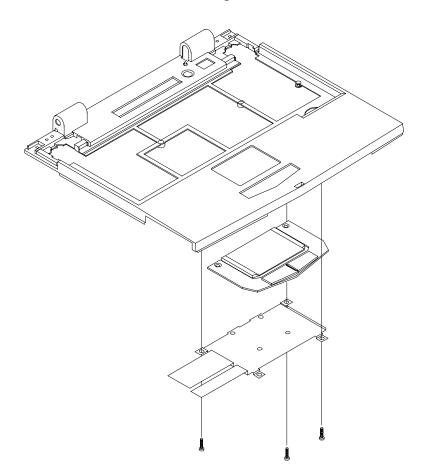
Figure 4-17 Removing the VersaGlide
