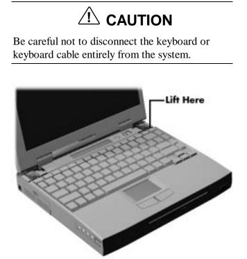
Figure 2-15 Lifting the Keyboard
