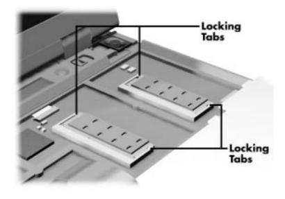
Figure 4-13 Removing an installed DIMM
