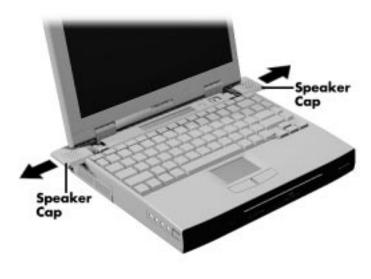
Figure 2-14 Removing the Speaker Caps
