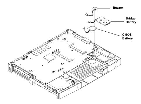
Figure 4-19 Removing Bridge Battery, CMOS Battery and Buzzer
