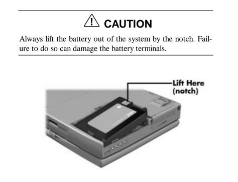
Figure 2-6 Removing the Battery
