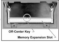
5. To install a memory module, insert the module into the expansion slot at an angle and then push it down until it clicks into place. To be certain that the module is installed correctly, ensure that the off-center notch on the module is aligned with the off-center key of the expansion slot. The module can only be installed one way due to the position of the notch.
