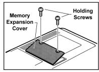
3. Locate the memory expansion cover on the bottom panel. Locate the two holding screws securing the cover to the bottom panel. Remove the screws with a small Phillips-Head screwdriver. Then remove cover by lifting up.
