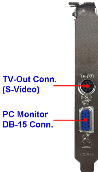
Figure 2-3. SILURO™ GF256 GTS graphics accelerator card plate layout.
