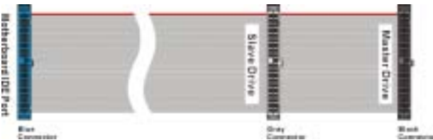
Figure 2-10. Ultra DMA 66 Ribbon Cable Outline
