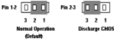
Figure 2-8. CCMOS1 jumper setting
