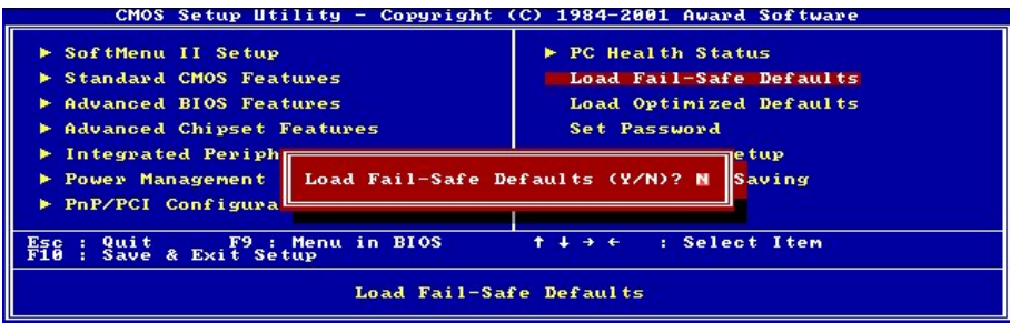
Figure 3-12. Load Fail-Safe Defaults Screen Shot
