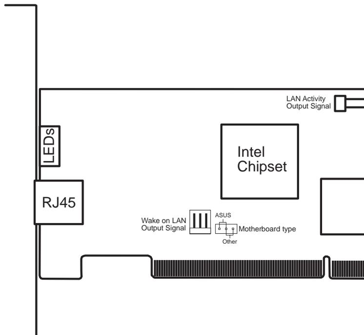
If you are using the ASUS PCI-L101 on an ASUS motherboard, leave the jumper on its default setting of “ASUS.” If you are using another brand of motherboard, set the jumper to “Other.” Connect the Wake on LAN (WOL) output signal to the motherboard’s WOL\_CON in order to utilize the wake on LAN feature of the motherboard. Connect the LAN activity output signal (LAN\_LED) to the system cabinet’s front panel LAN\_LED in order to display the LAN data activity.
