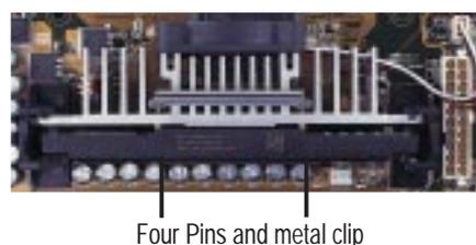
**NOTE:** The SEPP heatsink and fan (for Intel Celeron processors) is similar to the SECC2 heatsink and fan except that the clamping design is different.
