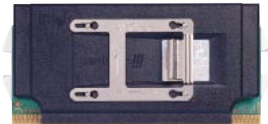
Example of an incorrectly installed retention clip
