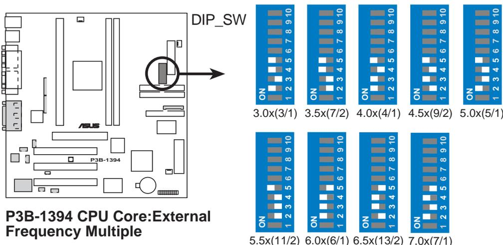
Set the DIP switches by the Internal speed of your processor as follows:
