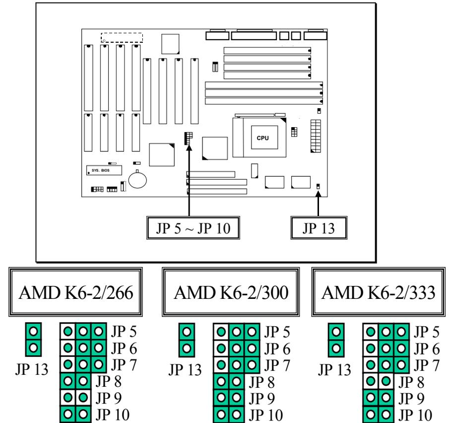
**NOTE:** JP13 is designed to support the 2.2V CPU Core voltage, When short connected, the CPU Vcore will be 2.2V and it will allow you to install the AMD K6-2 processors. If you are not using the AMD K6-2 processors, please leave JP13 open and refer to the manual for jumper settings.
