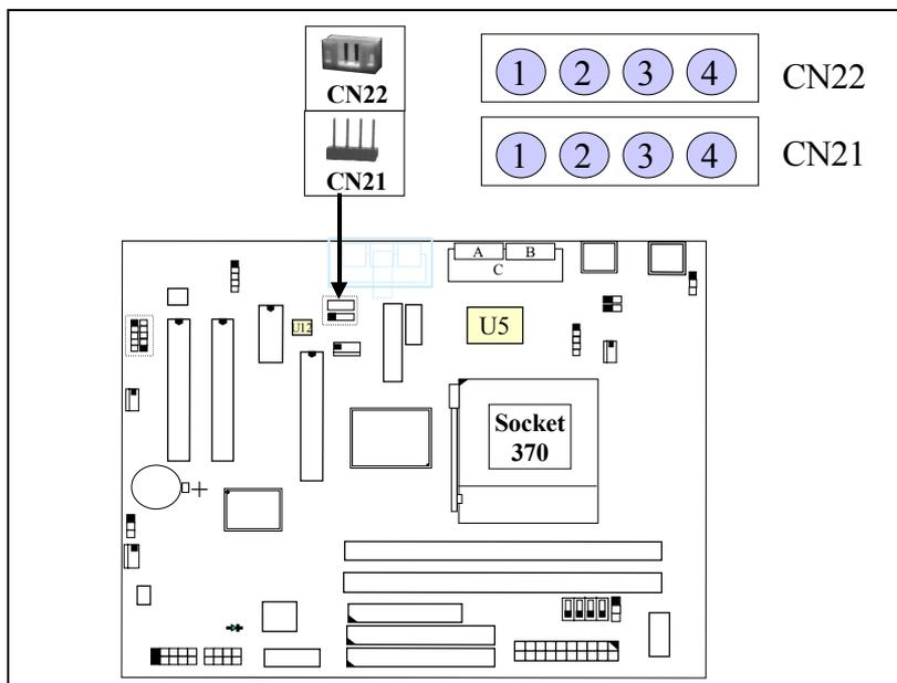
Note : You may find that there is the audio cable comes with the CD ROM drive. However, the pin assignment and outlook of the audio cable can be different from different vendors. There are two CD-IN connectors designed on the mainboard, which will meet most of the CD cable requirement. In case that you can not hear the CD audio output from the onboard audio interface, please refer to the following pin assignment of the CD-IN connector and make the proper audio cable connection:
