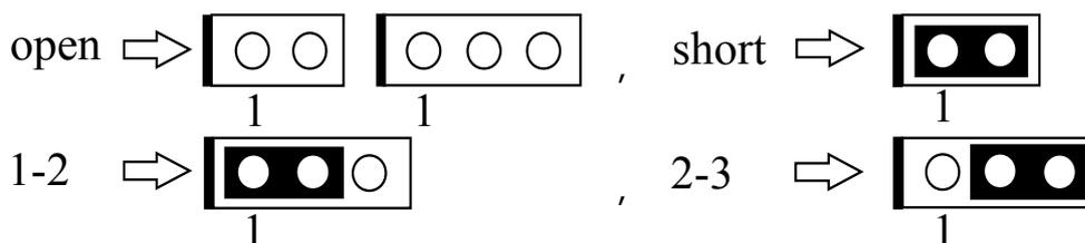
A jumper is a set of two, three or more jumper pins which allows users to make different system configuration by putting the plastic connector plug (mini-jumper) on it. The jumper setting is necessary when installing different components onto the mainboard.
