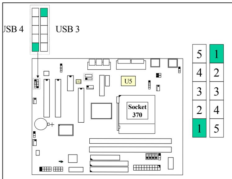
**3.3.28 CN32: USB 5 (Universal Serial Bus) Connector**
