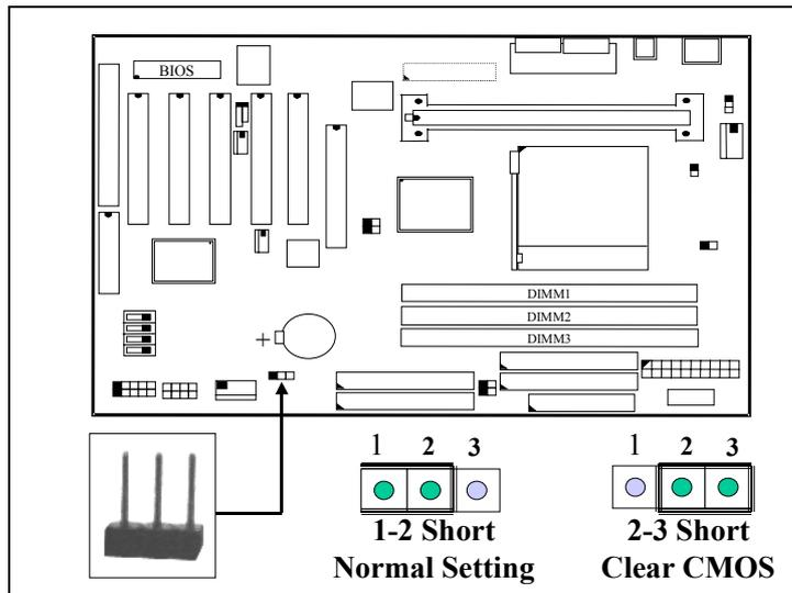
**Note:** JP9 is designed to clear the information which is stored in the CMOS memory. Improper connection on JP9 will cause mainboard failed to work. Please refer to the following steps to clear the CMOS
