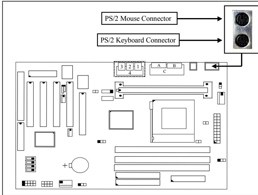
**(C) CN3 : Serial Port COM 1 Connector**
