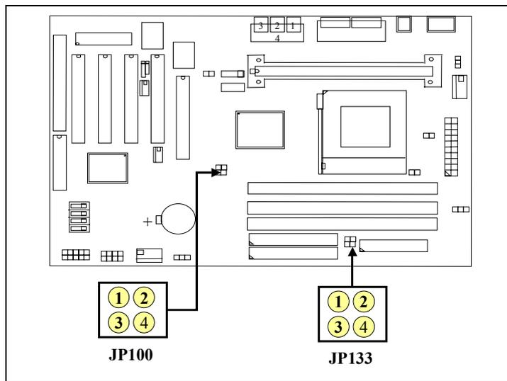
This mainboard is designed by using either VIA 693 or 693A chipset. When VIA693 is installed on the mainboard, you will see only JP100 on the board and you can use it to tell the mainboard to use the choosen FSB clock in the following table despite the CPU installed on the mainboard. If you found the VIA693A chipset installed on the mainboard, then you will see both JP100 and JP133 on the board and you can refer to the following table to select different FSB clock:
