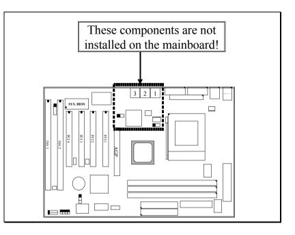
When you want to have the sound interface in your PC system afterward, you will have to purchase an ISA or PCI sound card and have it installed onto the mainboard. Before you can use that sound card, you will have to run the device driver which comes with the sound card so that the sound card will be working properly.
