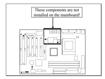
When you want to have the sound interface in your PC system afterward, you will have to purchase an ISA or PCI sound card and have it installed onto the mainboard. Before you can use that sound card, you will have to run the device driver which comes with the sound card so that the sound card will be working properly.
