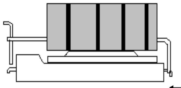
4. Push down the opposite side of the metal clip firmly and carefully to lock the cooler in place.
