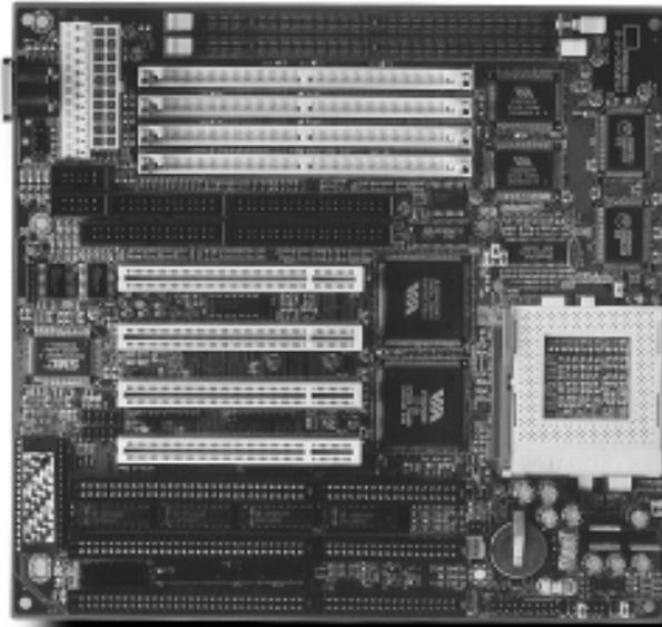
EFA Corporation of America is dedicated to offer performance, reliability, and flexibility in our system board designs. Designed and manufactured at our ISO 9001 compliant facilities, the Viking II system board offers a competitive socket-7 solution with the latest technologies. With support for the Ultra DMA 33 Protocol, SDRAM DIMMs, and flexible BUS speeds up to 75MHz, the Viking II offers all the amenities of a complete Socket-7 solution.
