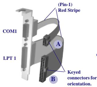
Serial (COM1) and Parallel (LPT1) cable assembly.
