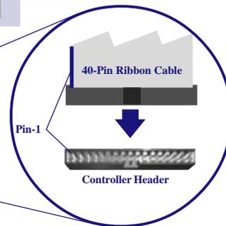
5. Locate pin-1 on the ATAPI device. (Note: pin-1 is usually located next to the power connector)
