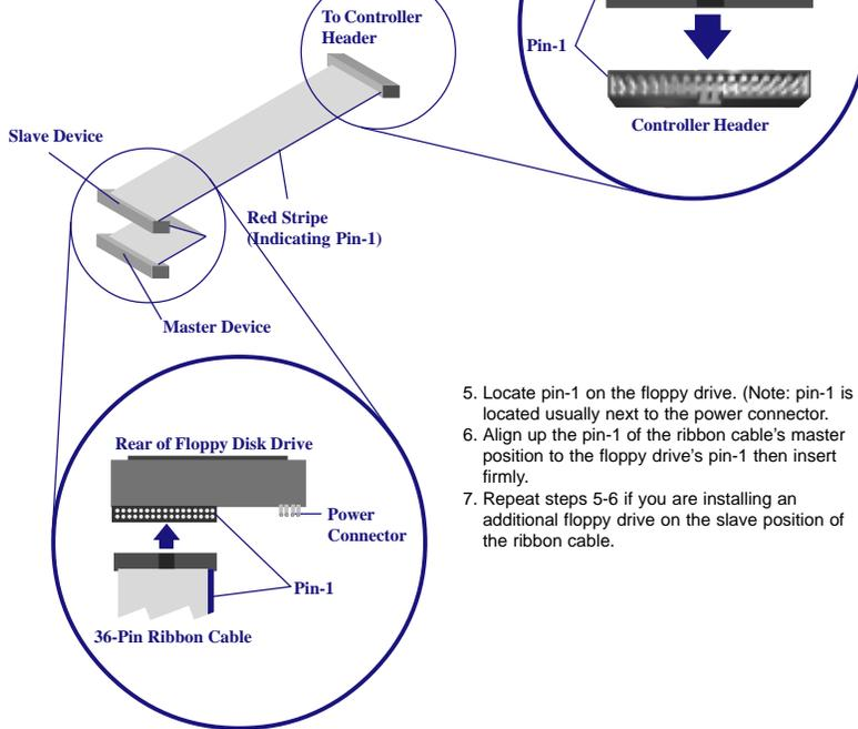
5. Locate pin-1 on the floppy drive. (Note: pin-1 is located usually next to the power connector.
