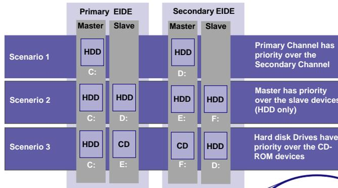
Fig A. Device Priority Diagram
