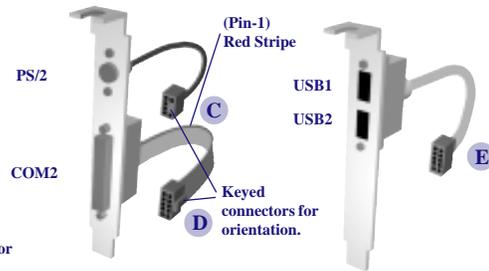
Serial (COM2) and PS/2 (BUS Mouse) cable assembly.
