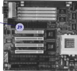
1. Note the location of the floppy disk drive controller header.
