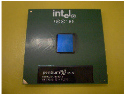
Figure 1: INTEL® Pentium® III Socket 370 Processor(FC-PGA)
