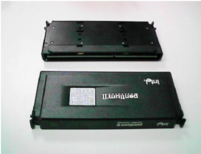
Figure 2:OEM Pentium® II Processor
