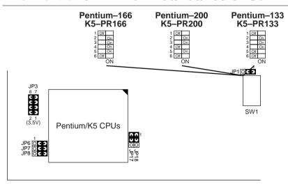
Figure 2–6. CPU Type Configuration
