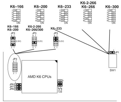
Figure 2–2. CPU Type Configuration
