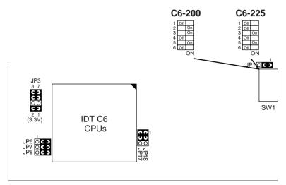
Figure 2–5. CPU Type Configuration
