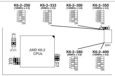
Figure 2–3. CPU Type Configuration
