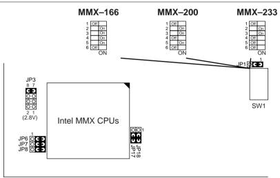
Figure 2–1. CPU Type Configuration
