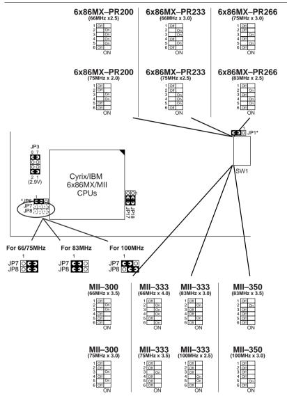
Figure 2-4. CPU Type Configuration
