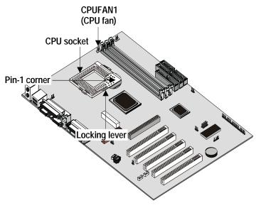
1. On the mainboard, locate the CPU socket and the CPU cooling fan CPUFAN1.
