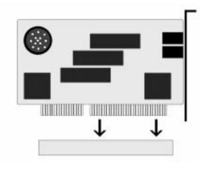
Figure 3-5: Installing an ISA Peripheral Card
