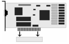
Figure 3-4: Installing a PCI Card
