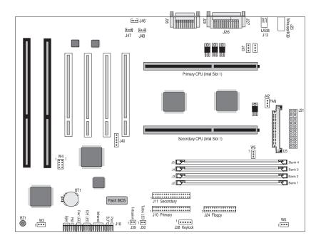
Figure 2-1. Dual Fortress System Board Diagram
