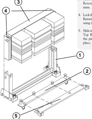
Figure 3-2: Installing a CPU
