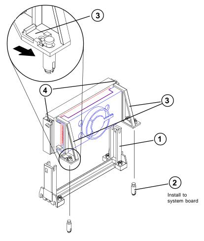
Figure 3-3: Installing a CPU (Boxed version)
