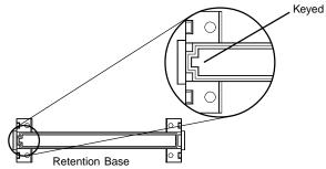
3. Using a screwdriver, tighten all four sides of the Retention Base.
