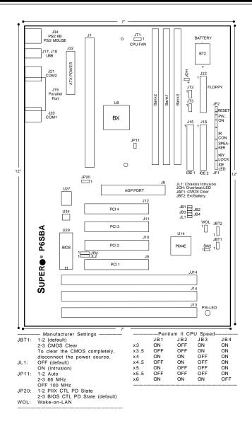
Figure 1-12. SUPER P6SBA Motherboard Layout
