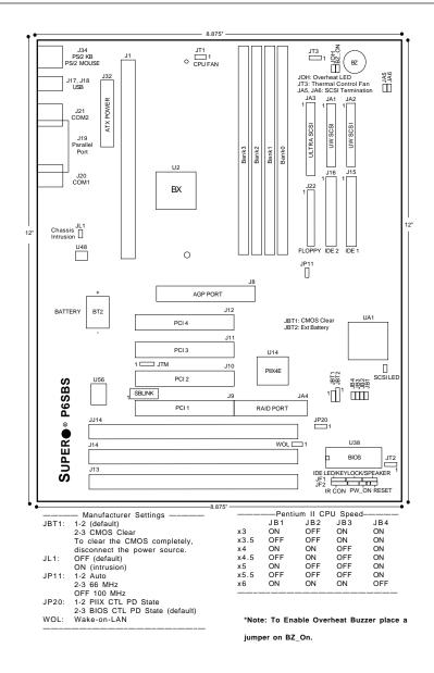
Figure 1-10. SUPER P6SBS Motherboard Layout
