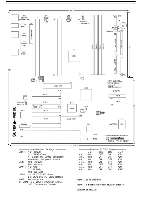
Figure 1-6. SUPER P6DBU Motherboard Layout
