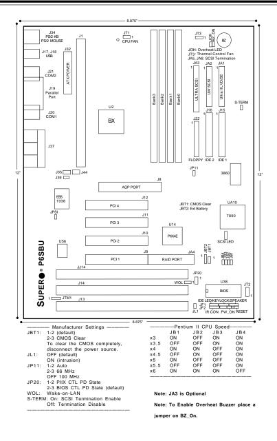
Figure 1-8. SUPER P6SBU Motherboard Layout
