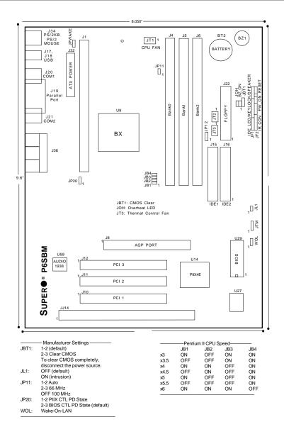
Figure 1-14. SUPER P6SBM Motherboard Layout
