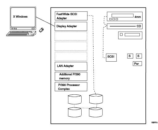
Figure 10. RISC/6000-591 S/390 Basic Configuration. There is not a "standard" configuration for a basic OS/390 system. This illustrates an entry configuration that would serve for basic OS/390 usage. The disk drives would probably be 2.25 GB units, although you have a choice of drives. See Chapter 3, "Installation" on page 43 for a discussion of the amount of disk space needed.
