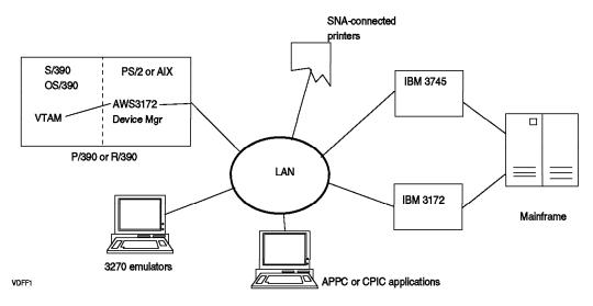
Figure 21. LAN SNA Connections. A variety of SNA connections are possible over a LAN, including full SNA interoperability with a mainframe.
