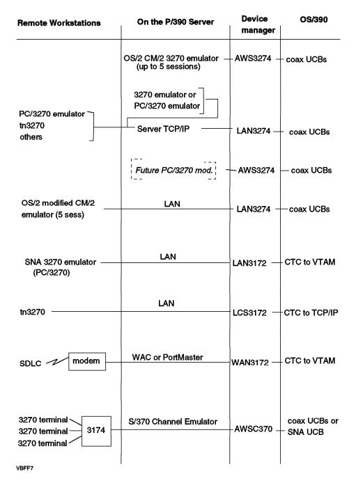
Figure 12. Methods of Connecting 3270 Terminals to the P/390
