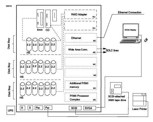
Figure 7. PC Server System/390 Configured for Additional Disks. A PC Server 520 is the base unit.
