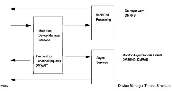
Figure 3. General Thread Structure for Device Manager
