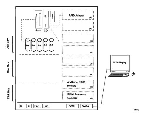
Figure 4. Basic PC Server System/390 for OS/390. This is the base configuration of a system intended for use with OS/390. Use with OS/390 implies that the additional P/390 memory "daughter card" is installed, and five 2.25 GB disk drives are installed. Later versions of the P/390 may use the planar SCSI adapter for the 4mm tape and the CD-ROM drive.
