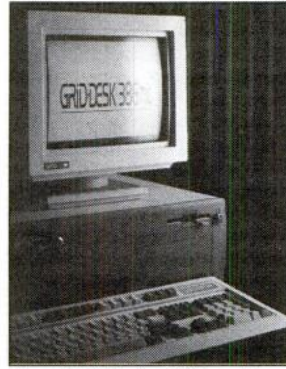
The Grid-Desk 386mc is a Micro Channel desktop PC with 2 megabytes of RAM.
