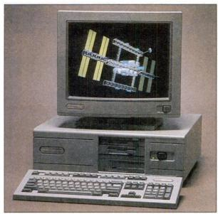
At an estimated performance rating of 5 MIPS, Compaq's Deskpro 386/33 with 64K of cache is a third faster than its 25-MHz model.
