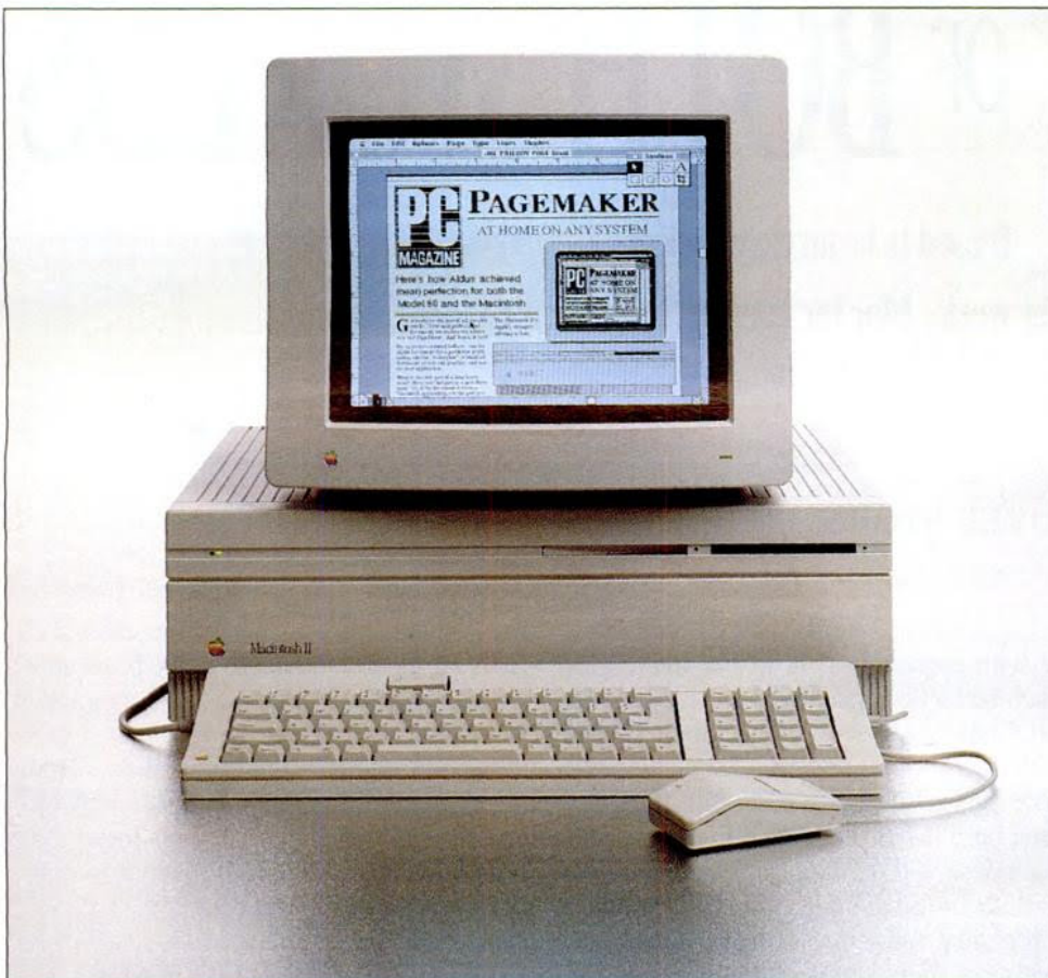
The Macintosh II looks more like an AT-compatible machine than the familiar one-piece unit from which it has evolved. The full-size (13-inch) color monitor, a feature long desired by Mac users, offers the same kind of Macintosh high resolution that has always awed PC users.
