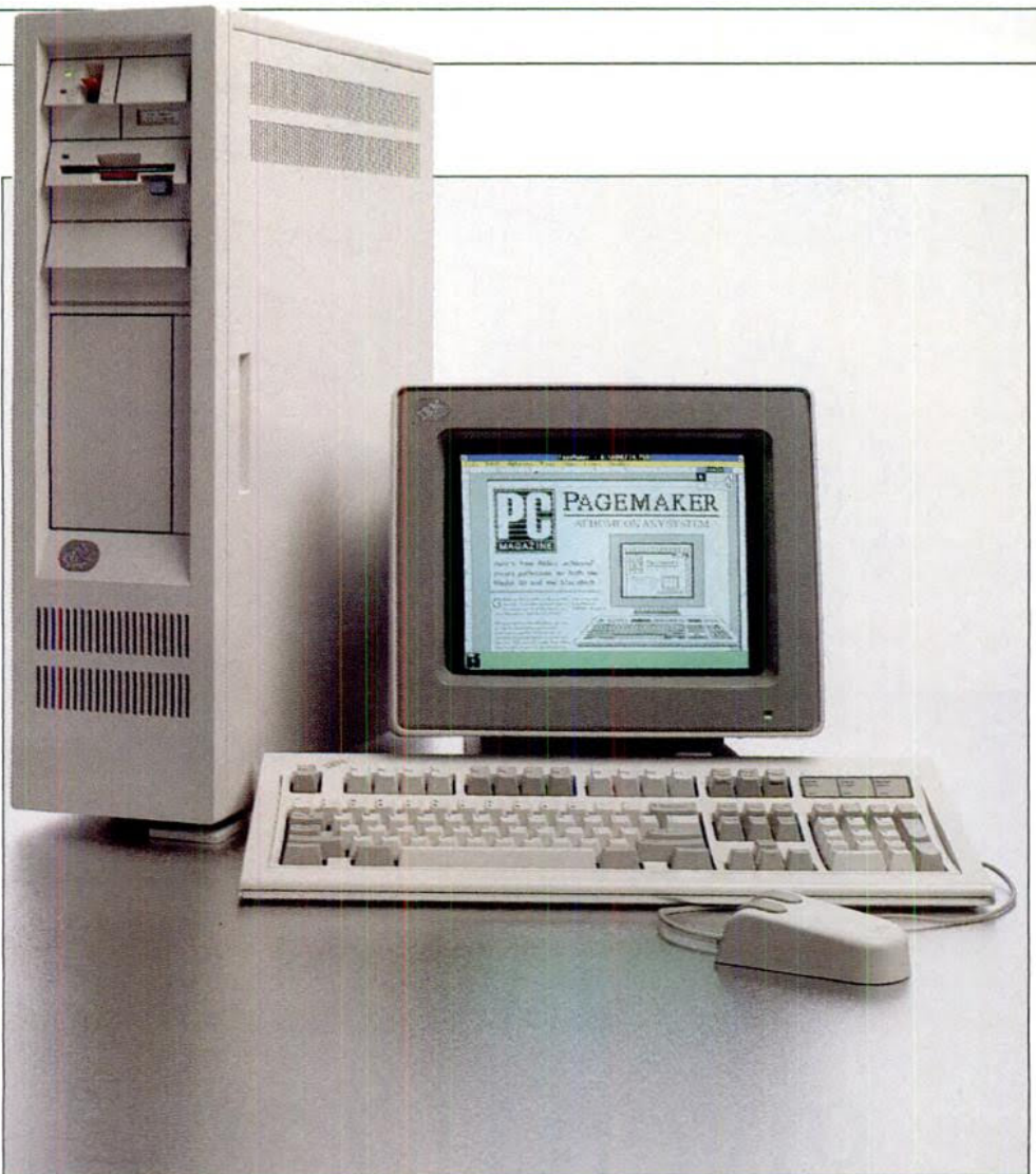
As the flagship of the PS/2 family, the IBM PS/2 Model 80 provides 80386 processing power, and VGA resolution circuitry, which is built into the motherboard, allows the monitor to generate high levels of resolution and 16 of 256 colors on-screen.
