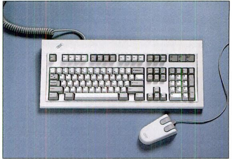
The 101-key IBM Enhanced keyboard is standard with the PS/2 Model 80. Its solid feel and audible and tactile feedback remain unmatched by any other keyboard. It has 12 function keys.
