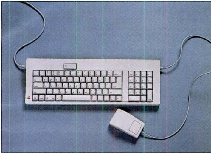
The 81-key Macintosh Plus-style keyboard that comes standard with the Macintosh II has no function keys but does have a unique power on/off button located at the top center.
