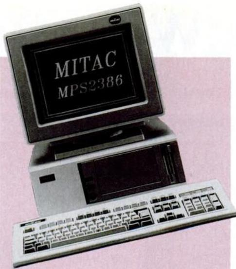
American Mitac's 386SX-based MPS2386 computer features Micro Channel architecture.
