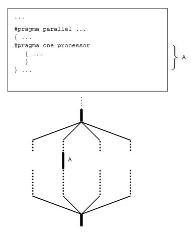
Figure 5-6 One Processor Segment
