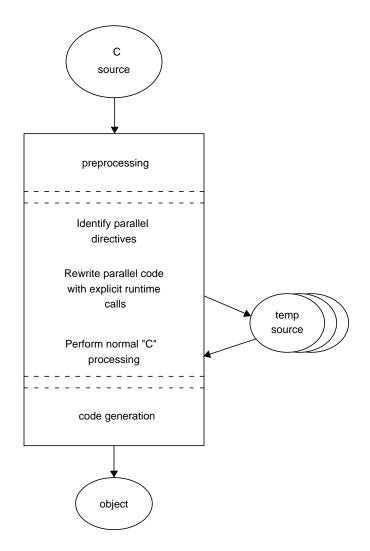
Figure 2-3 Multiprocessing Compiler Flow
