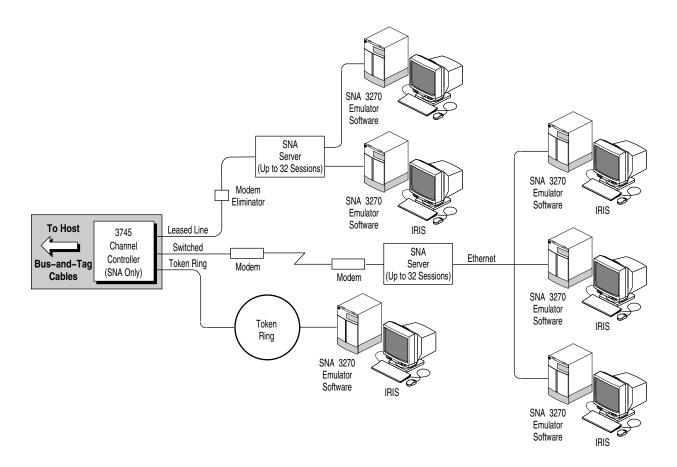
Figure ii 3270 Emulator with IBM 3745 Channel Controller
