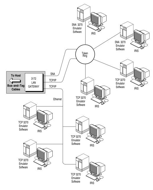
Figure iii 3270 Emulator with IBM 3172 LAN Gateway
