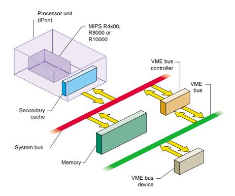
Figure 12-1 Relationship of VME Bus to System Bus
