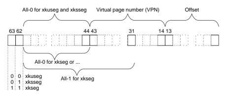
Figure 1-9 MIPS 64-Bit Virtual Address Format
