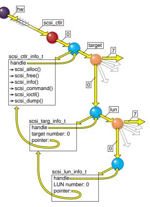
Figure 16-1 SCSI Vertexes and Data Structures
