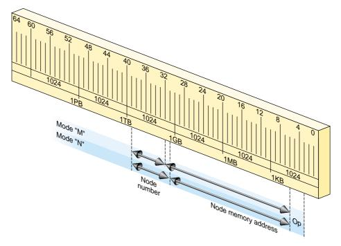
Figure 1-12SGI Origin 2000 Fetch-and-Op Address Decoding
