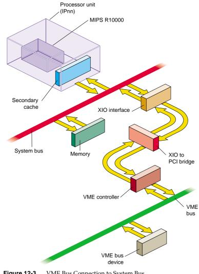
Figure 12-3 VME Bus Connection to System Bus
