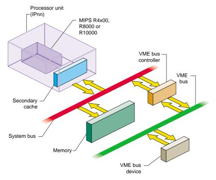
Figure 14-1 Relationship of VME Bus to System Bus
