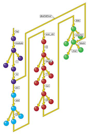
**Figure 2-1** Part of a Typical Hwgraph
