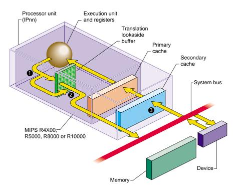
Figure 1-2 CPU Access to Device Registers (Programmed I/O)
