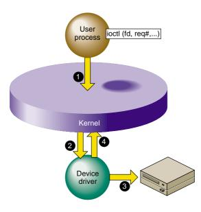
Figure 3-2 Overview of Device Control
