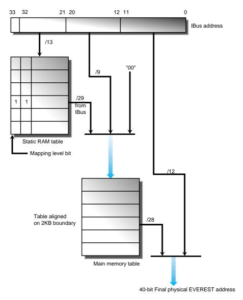
Figure 14-3 I/O Address to System Address Mapping
