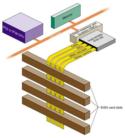
Figure 18-1 High-Level Overview of EISA Bus in Indigo<sup>2</sup>
