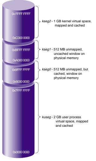
Figure 1-5 The 32-Bit Address Space
