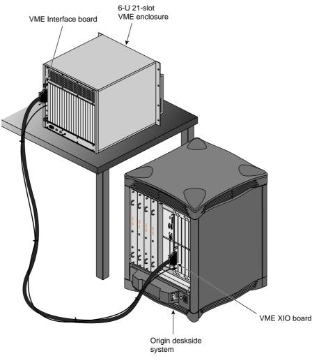
Figure 12-2 VME Bus Enclosure and Cable to an Origin 2000 Deskside
