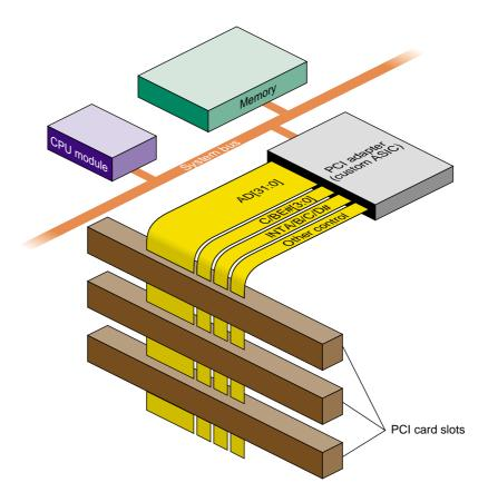
Figure 20-1 PCI Bus In Relation to System Bus
