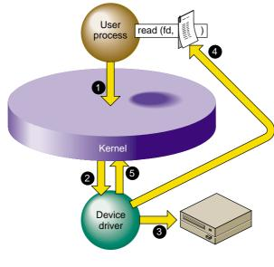
Figure 3-3 Overview of Programmed Kernel I/O
