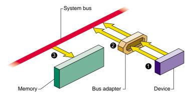
Figure 1-4Device Access Through a Bus Adapter
