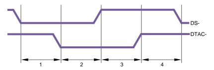
Figure 14-4VMECC Contribution to VME Handshake Cycle Time
