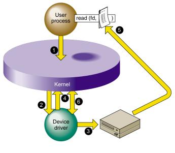
Figure 3-5 Overview of DMA I/O
