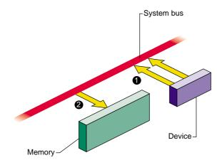
Figure 1-3 Device Access to Memory
