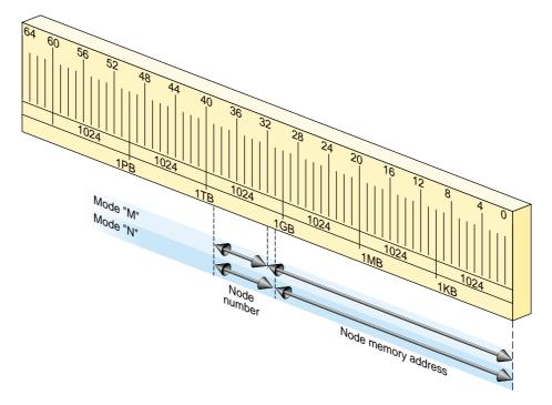
Figure 1-11 SGI Origin 2000 Physical Address Decoding
