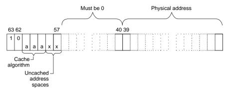
Figure 1-10 Address Decoding for Physical Memory Access
