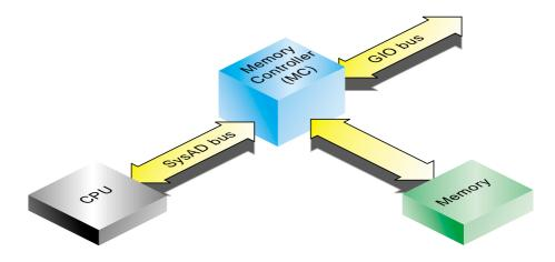
Figure 19-1 The SysAD Bus in Relation to GIO
