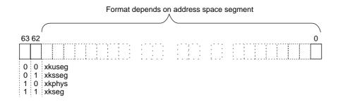
Figure 1-8 Selecting the MIPS 64-Bit Address Space Segments
