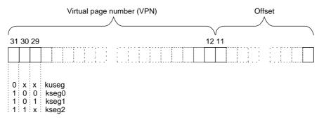
Figure 1-6 MIPS 32-Bit Virtual Address Format
