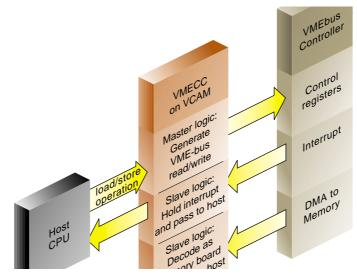
Figure 14-2 VMECC, the VMEbus Adapter
