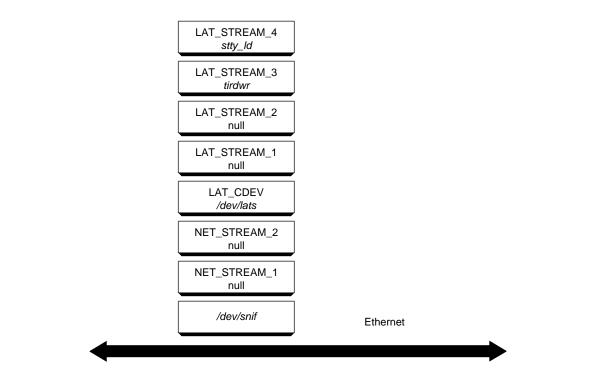
Figure 2-2 The STREAMS Stack for 4DLT
