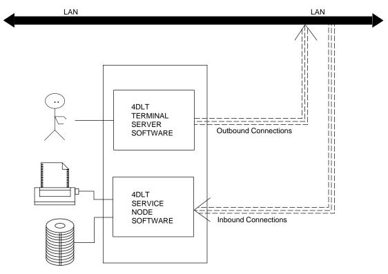
Figure 1-1 LAT Functions on a 4DLT Node
