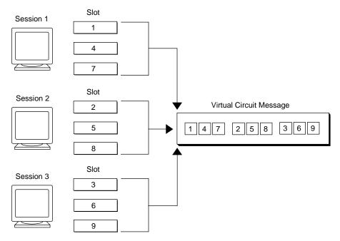
Figure 1-6 Multiplexing Slot Data into a Virtual Circuit Message
