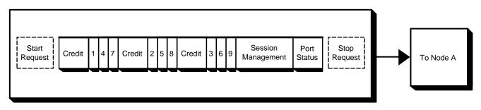
Figure 1-7 Virtual Circuit Message Components
