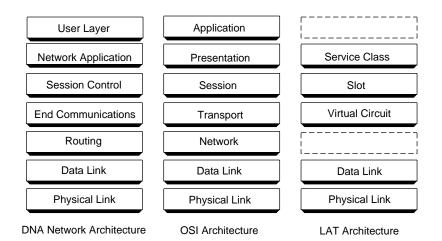
**Figure 1-4** LAT Protocols Compared to the DNA and OSI Models
