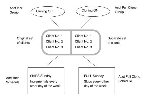
Figure 5-12 Automatic Cloning Scheme
