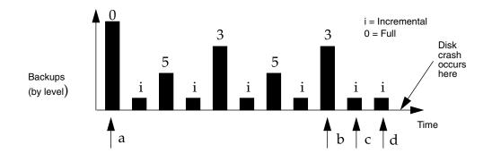
Figure A-1 Backups Needed for Disaster Recovery
