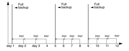
Figure 2-6 Full Versus Incremental Backups
