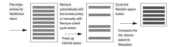
Figure 2-11 Reclaiming Space From the Index
