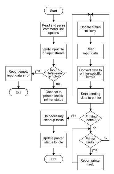
Figure 3-1 Printer Driver Processing Overview
