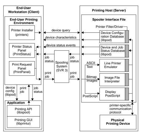
Figure 1-1 Impressario Printing Architecture
