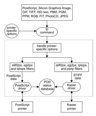
Figure 1-3 General Filter/Driver Architecture
