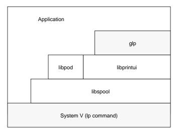
Figure 1-4 System V Spooling System Interface
