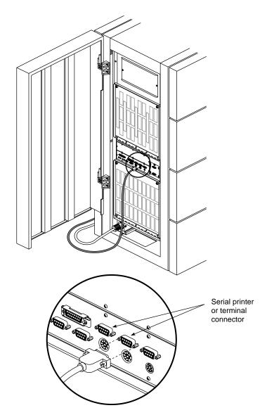
**Figure 4-9** Connecting a Serial Printer or ASCII Terminal
