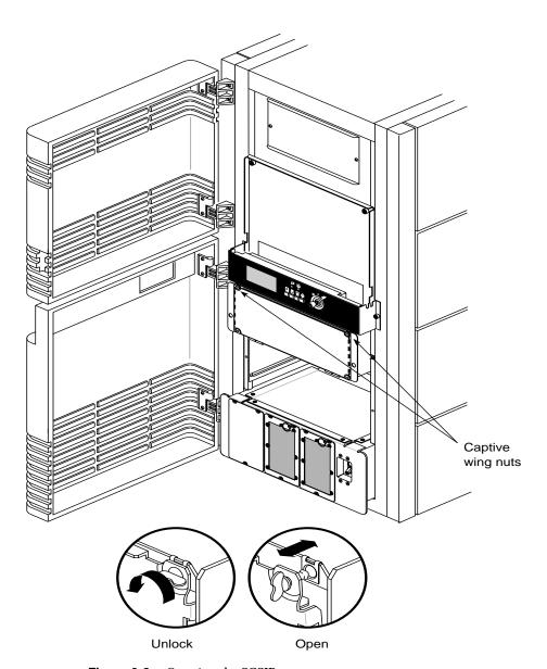
**Figure 3-8** Opening the SCSIBox
