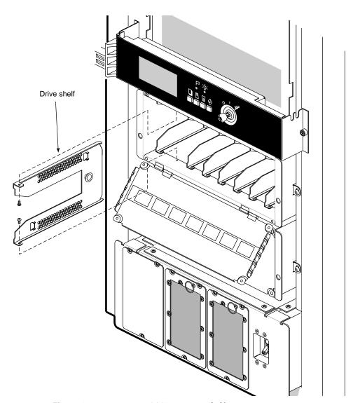
Figure 4-3 Removing a SCSIBox Drive Shelf
