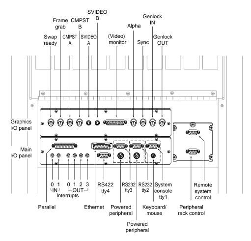
Figure 2-5 Main and Graphics I/O Panel Connectors
