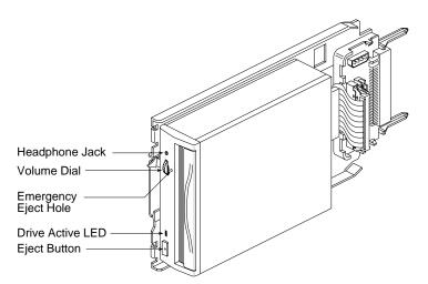
Figure 4-8 CD-ROM Front Panel Controls
