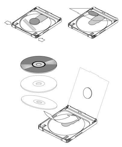
Figure 4-6 Loading a CD Into the Caddy
