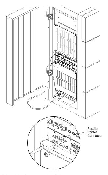
Figure 4-10 Connecting a Parallel Printer
