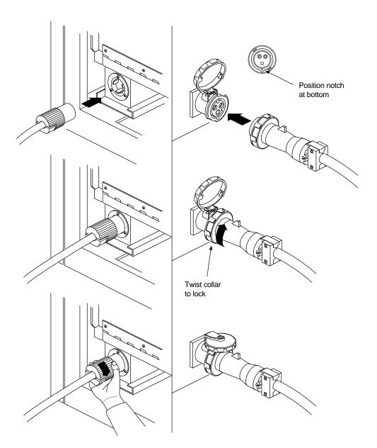
**Figure 3-10** Connecting the System Power Cable
