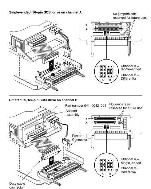
Figure 4-1 Channel Adapter Settings (Different Channel Configurations)
