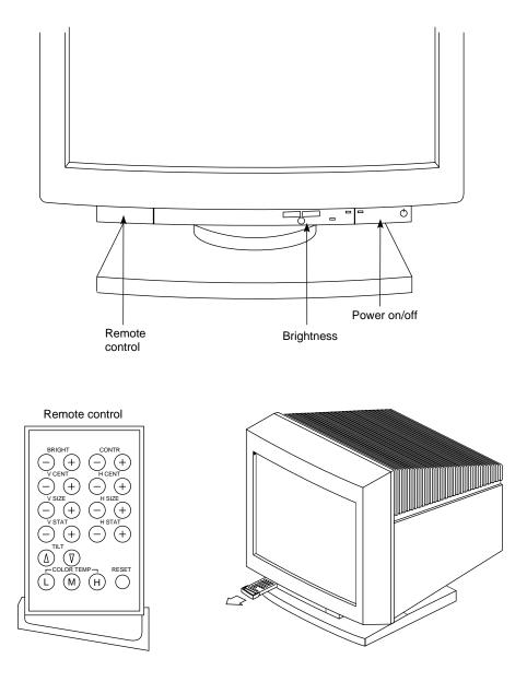
Figure 3-4 20-Inch Monitor Controls
