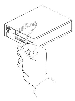
Figure B-3 Tape Head Cleaning
