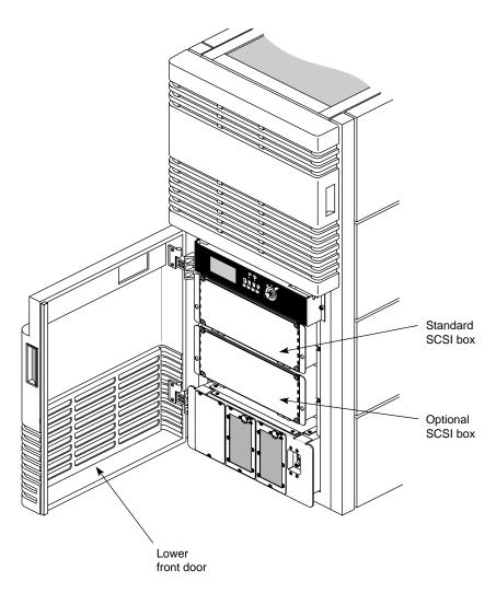
Figure 2-10 SCSIBox Drive Enclosures
