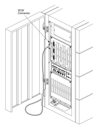
Figure 4-4 Connecting an External SCSI Device
