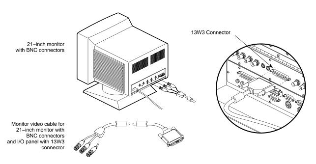
Figure 3-2 21-Inch Monitor Cable Connection
