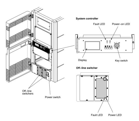
**Figure 2-3** Power Switches and Indicators
