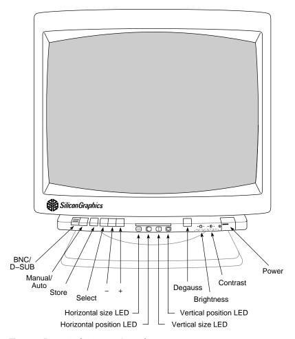
Figure 3-5 21-Inch Monitor Controls
