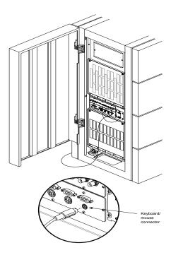
Figure 3-7 Keyboard Connection
