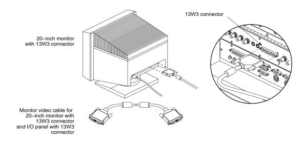
Figure 3-3 Connecting the 20-Inch Monitor
