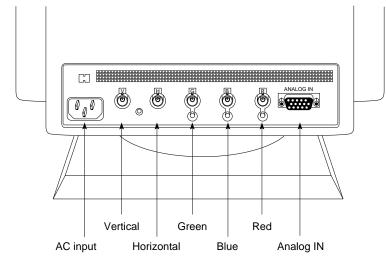
Figure 3-1 21-Inch Monitor Connectors
