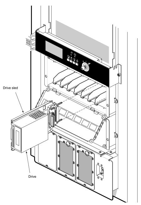
Figure 3-9 Installing a Front Loading Device
