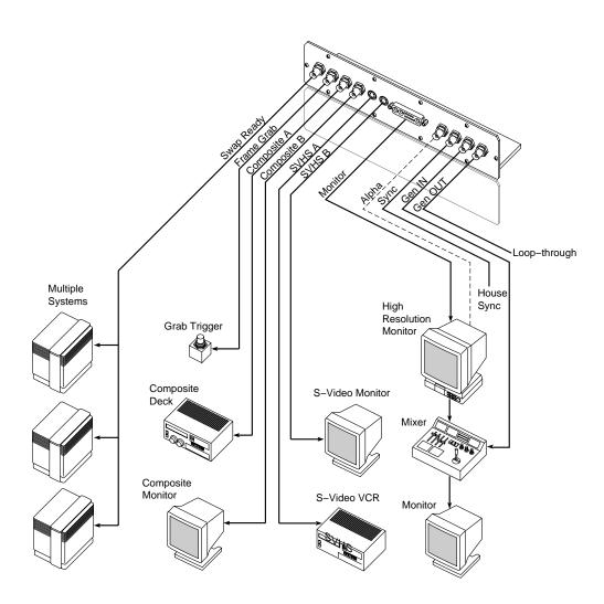
Figure 3-6 Typical Video Peripheral Configuration
