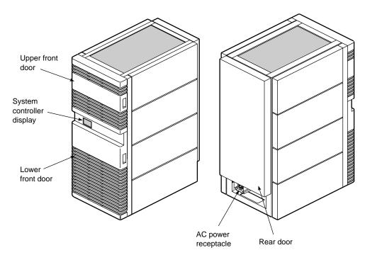
Figure 2-1 Chassis Front and Rear Views
