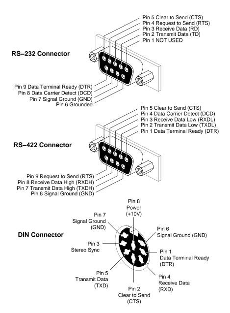
Figure 2-7 Powered and Unpowered Serial Connectors
