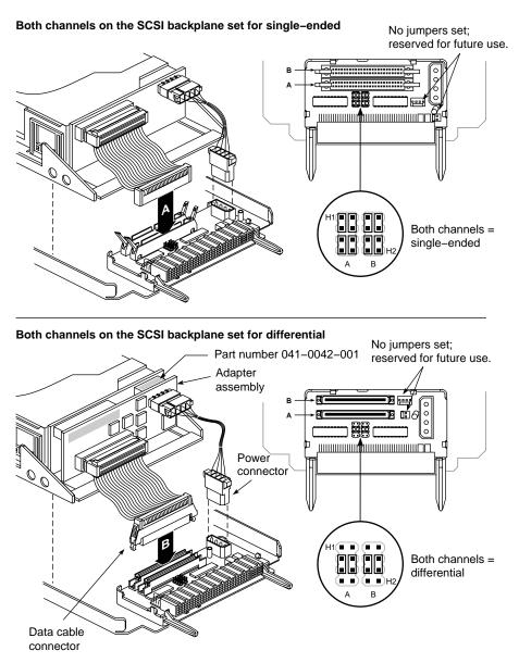
Figure 4-2 Channel Adapter Settings (Same Channel Configurations)
