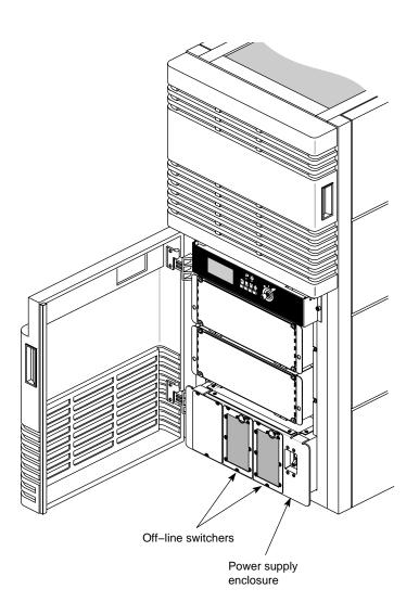
**Figure 2-11** Power Supply Enclosure with Three OLSs
