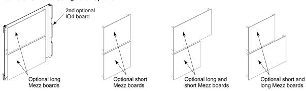
Figure D-3 Optional Second and Third IO4 Configuration
