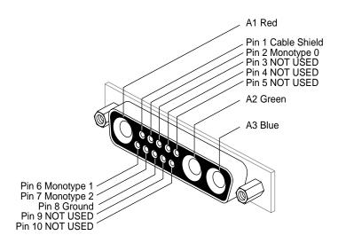
Figure 2-8 Video Monitor Connector Pinouts
