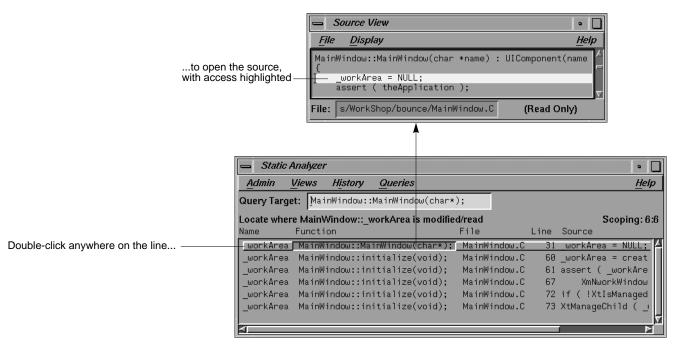
Figure 6-10 Query Result in Static Analyzer and Source View
