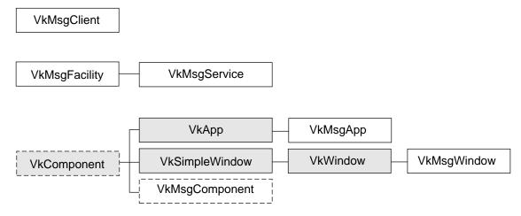
Figure A-1 The Inheritance Graph for the ViewKit Message Facility Classes
