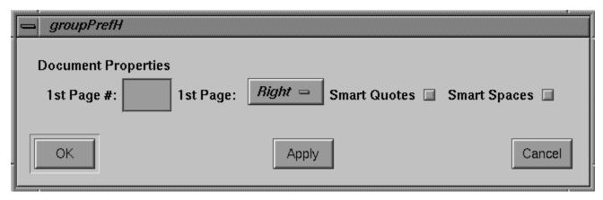
Figure 8-10 Example of a Horizontal VkPrefGroup Item with Label
