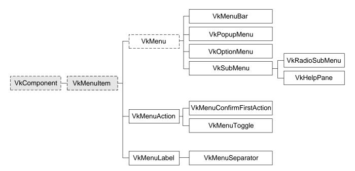
Figure 5-1 The Inheritance Graph for the ViewKit Menu Classes
