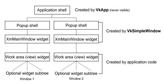
Figure 4-2 Widget Hierarchy of Top-Level Windows in ViewKit Applications
