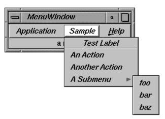
Figure 5-4 A Menu Pane Containing a Label and a Submenu
