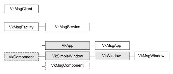
Figure A-1 The Inheritance Graph for the ViewKit Message Facility Classes
