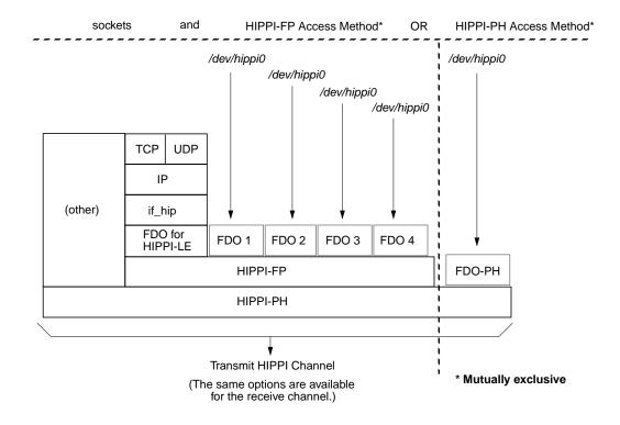
Figure 1-1 Interfaces for Controlling One Channel of the HIPPI Subsystem
