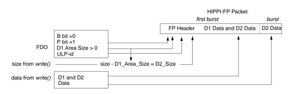
Figure 1-8 Single-Write HIPPI-FP Packet With D1 Data
