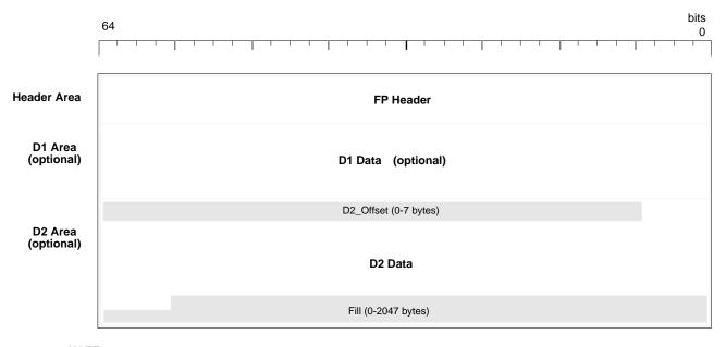
**NOTE:** The size of each included area must be an integral number of 64-bit words. The first word of each area must be 8-byte aligned.
