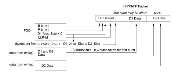
Figure 1-10 Multiple-Write HIPPI-FP Packet: Separate FP Header and D1 Data
