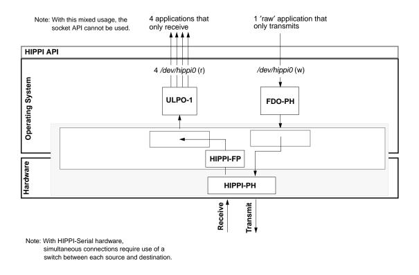
Figure 1-11 Block Diagram for Mixing HIPPI-PH and HIPPI-FP
