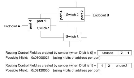
Figure 1-8 Routing With Source Addressing
