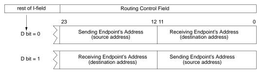
Figure 1-3 Routing Control Field With Logical Addressing
