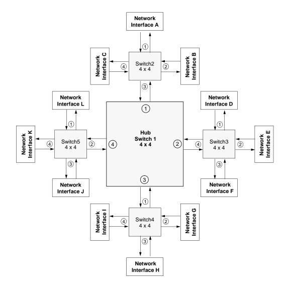
Figure 1-19 HIPPI LAN Configurations With Multiple Switches
