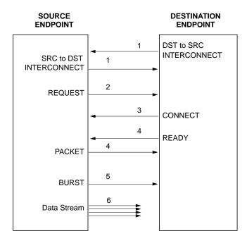
Figure 1-15 HIPPI Signals Used on Each Point-to-Point Link
