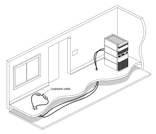
Figure 3-2 Installing a Loopback Link Using a Loopback Cable
