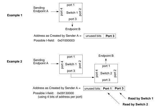
Figure 1-7 Port Identifiers for Source Addressing
