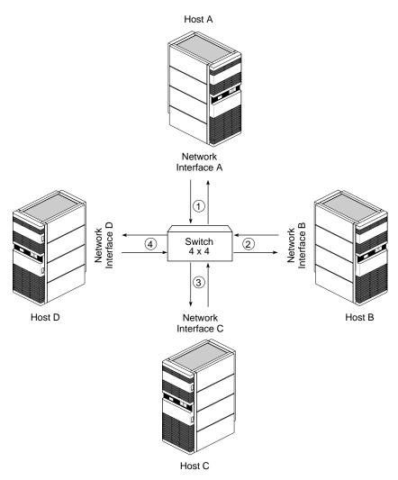
Figure 1-18 HIPPI LAN Configuration With One Switch
