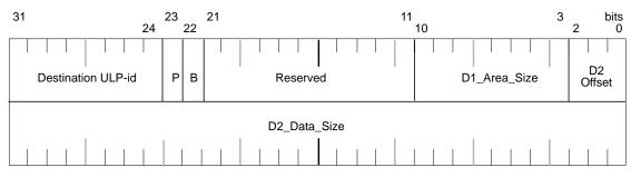
The 64-bit FP header describes the HIPPI packet using six fields, illustrated in Figure 1-12 and described in Table 1-4.
