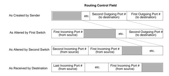
Figure 1-9 How Switches Alter Source Addresses
