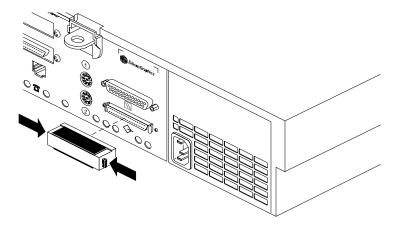
**Figure 6-5** Removing the 50-Pin SCSI Terminator From the Challenge S Server
