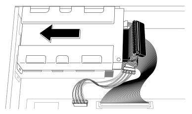
**Figure 6-4** Installing a Second Drive Above the System Disk
