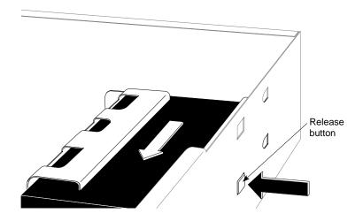
**Figure 9-24** Removing the System Disk Drive
