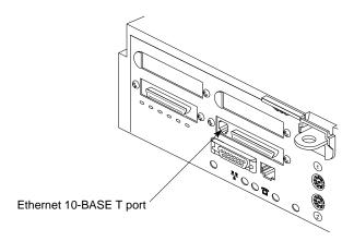
**Figure 3-5** Connecting an Ethernet 10-BASE T Cable to the Challenge S Server (S-100 and S-150 Models)
