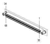
Figure A-7 68-Pin SCSI (High-Density) Pinout Numbering
