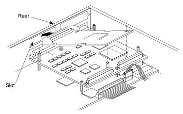
**Figure 5-3** Inserting the GIO Board's I/O Connector Through the Backplane
