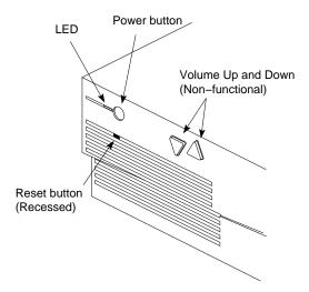
**Figure 2-3** Challenge S Front-Panel Controls
