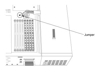
Figure 8-2 Locating the Password Jumper
