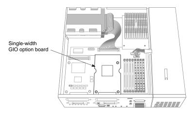
Figure 9-18 GIO Board Installed in Slot 0
