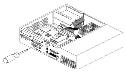
**Figure 9-5** Removing the Screw From the Connector on the Rear of the Server
