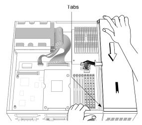
Figure 9-30 Installing the Power Supply
