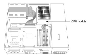
Figure 9-11 Locating the CPU Module
