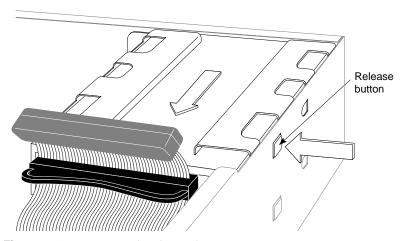
Figure 9-20 Removing the Floptical Drive
