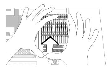
Figure 9-13 Disconnecting the CPU Module
