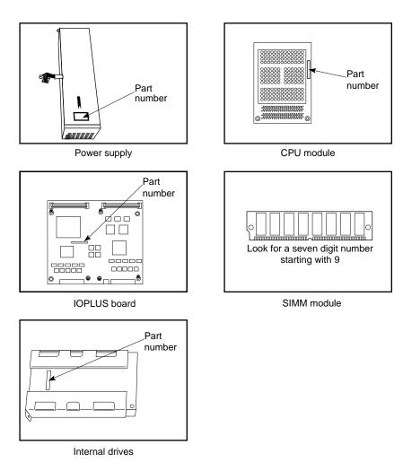
Figure 9-1 Part Number Locations for Standard System Components
