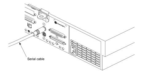
Figure 6-11 Connecting the Serial Cable to the Serial Port
