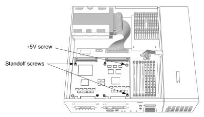
Figure 9-9 Removing the Screws From an IOPLUS
