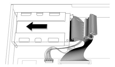
Figure 9-26 Installing the Replacement System Disk Drive
