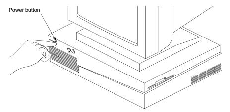
**Figure 3-8** Turning On the Challenge S Server
