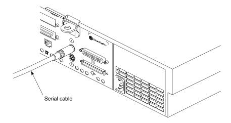
**Figure 3-2** Connecting the System Console (ASCII Terminal)
