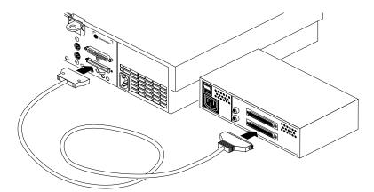
**Figure 6-6** Connecting an External 50-Pin SCSI Device to the Challenge S Server
