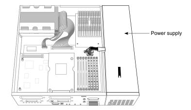
Figure 9-28 Locating the Power Supply
