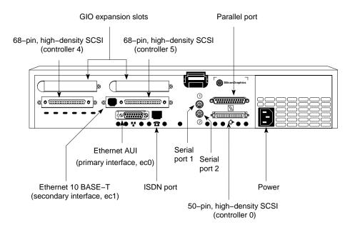
Figure 2-4 Challenge S Back-Panel Connectors
