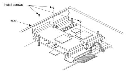
Figure 5-4 Installing a single-width GIO option board
