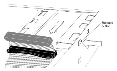
Figure 6-2 Removing An Internal Drive Bracket
