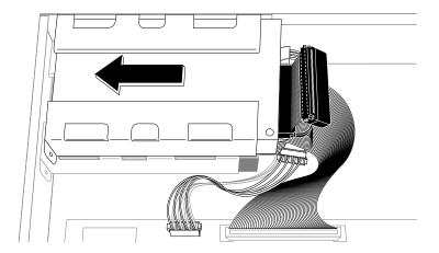
Figure 9-27 Re-installing the Floptical Drive
