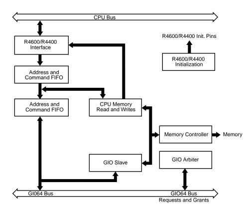
Figure 2-8 A Block Diagram of the MC1 ASIC
