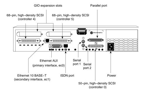
**Figure 3-1** Challenge S Back Panel Connectors
