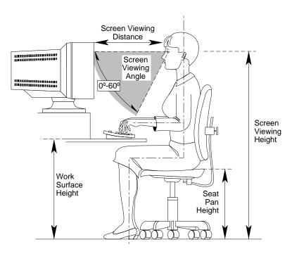
**Figure 10-1** Basic Parameters of Visual Display Terminal Workstation Adjustment (Adapted From ANSI/HFS 100-1988)
