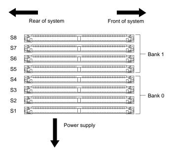
Figure 2-9 SIMM Bank and Slot Arrangement
