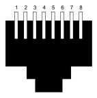
**Figure A-3** Ethernet 10-BASE T Pinout Numbering
