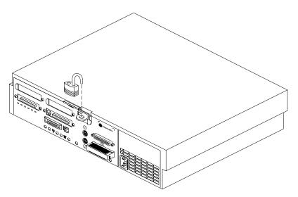
Figure 3-12 Attaching a Lock to the Challenge S Server
