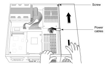
Figure 9-29 Removing the Power Supply
