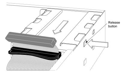
Figure 2-6 Example Drive Release Button
