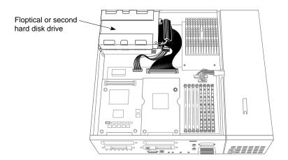
Figure 9-19 Locating the Floptical or Second Hard Disk Drive
