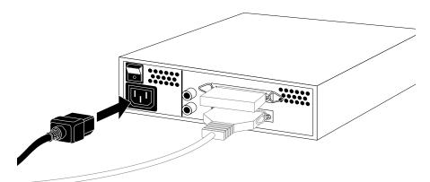
Figure 6-9 Connecting the Power Cable to an External Device
