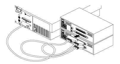
Figure 6-7 Daisy-Chaining an External 50-pin Single-Ended SCSI Device
