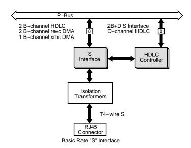
Figure 2-11 ISDN Interface Architecture.
