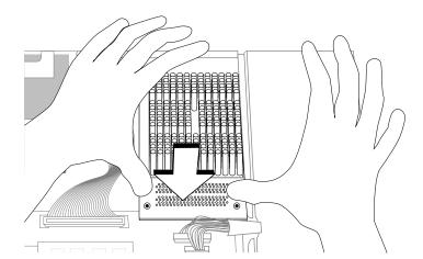
Figure 9-14 Installing the CPU module
