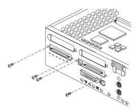
**Figure 9-8** Removing the Screws From the IOPLUS Board's I/O Connector
