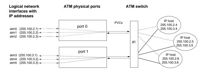
Figure 1-23 IP-over-PVC Configurations That Do Not Conform to RFC 1577
