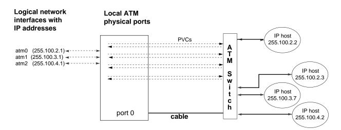
Figure 1-22 Multiple IP Interfaces Using a Single ATM Physical Port With PVCs
