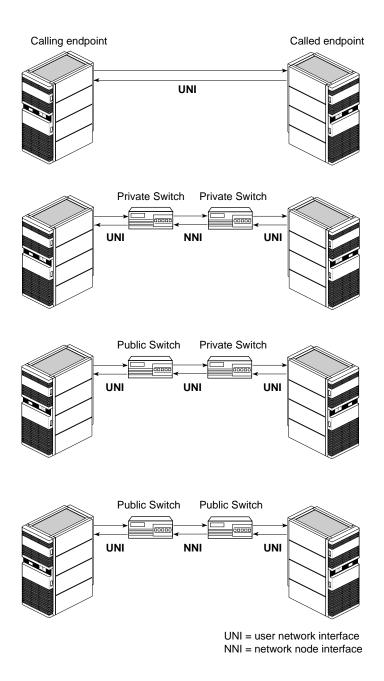
Figure 1-14 Use of UNI and NNI Protocols for ATM Signalling
