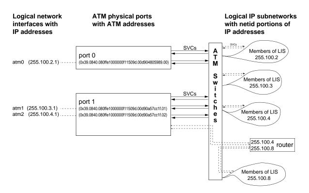
Figure 1-21 Multiple IP Interfaces Using Each ATM Physical Port With SVCs
