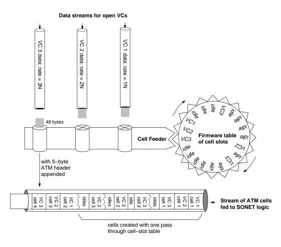
**Figure 1-25** Transmission Rate Control on ATM-OC3c XIO Board for Origin and Onyx2 Platforms
