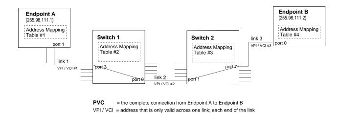
Figure 1-12 General Overview of PVC Configuration Tasks
