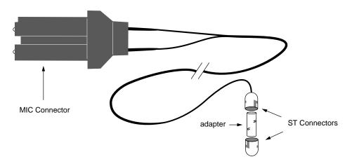
Figure 2-2 Loopback Cable Assembly and Adapter for MIC Connector
