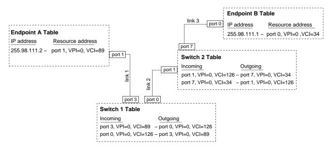
Figure 1-13 Example of Address Mapping Tables for One PVC
