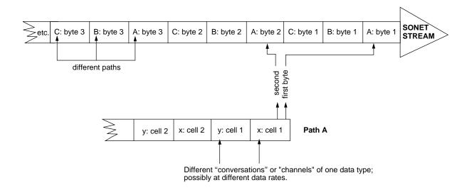
Figure 1-6 Byte-multiplexing Within a SONET Stream
