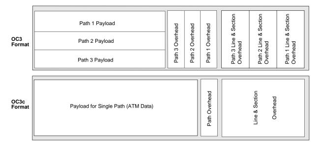
Figure 1-8 SONET OC3 versus OC3c Frame Format
