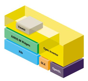
Figure 1-1 How X, OpenGL, and Toolkits Are Layered
