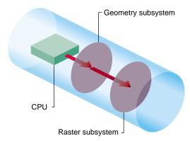
**Figure 13-1** Three-Stage Model of the Graphics Pipeline
