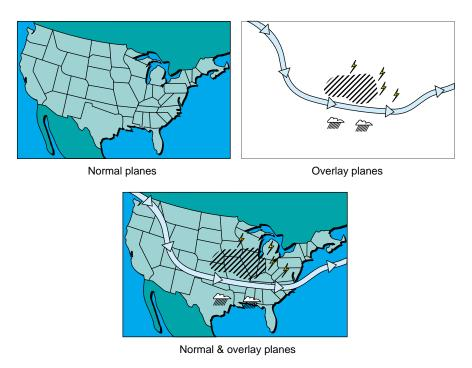
Figure 4-1 Overlay Plane Used for Transient Information
