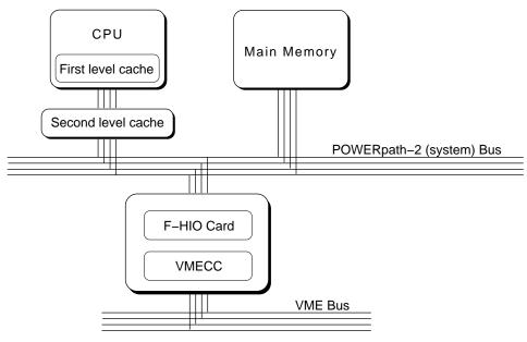
Figure 6-1 Multiprocessor Challenge Data Path Components
