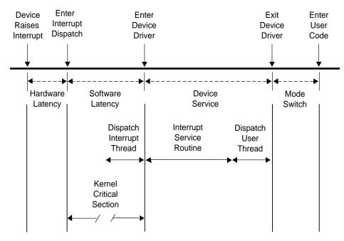
**Figure 3-2** Components of Interrupt Response Time
