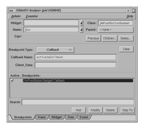
Figure 11-4 Setting Breakpoints for a Widget Class
